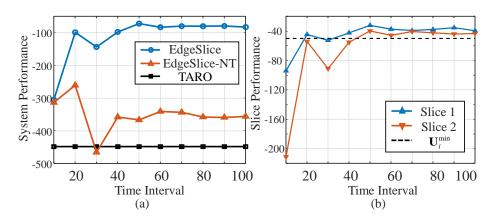
Figure 7.5: The convergence of algorithms: (a) system performance vs. time interval; (b) slice performance vs. time interval.
