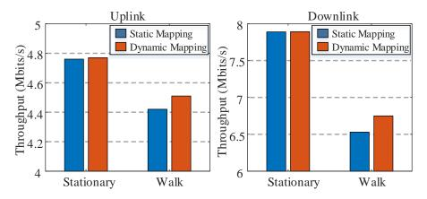
Figure 5.6: The comparison between static and dynamic mapping.
