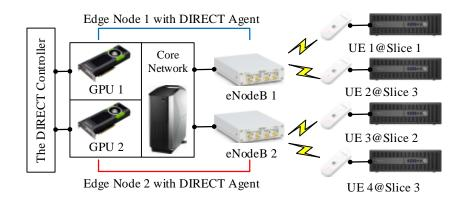
Figure 6.5: The testbed implementation of DIRECT protocol.
