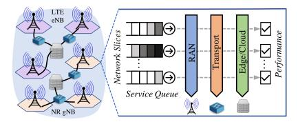
Figure 1.5: An illustration of end-to-end network slicing.
