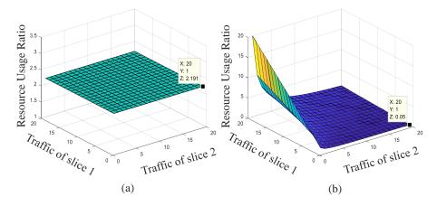
Figure 7.8: The performance of orchestration agents: (a)  $\eta_1/\eta_2$  vs. slice traffic under EdgeSlice-NT; (b)  $\eta_1/\eta_2$  vs. slice traffic under TARO.
