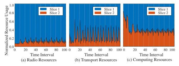
Figure 7.6: The multiple resource orchestrations of EdgeSlice: (a) radio resource; (b) transport resource; (c) computing resource.
