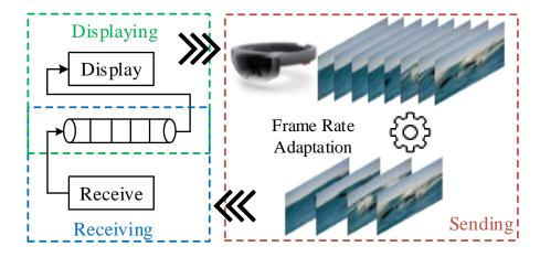
Figure 3.6: Frame rate adaptation and transceiving pipeline.
