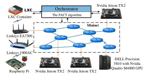
Figure 4.9: The edge-base MAR testbed.
