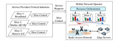
Figure 1.4: Distributed network slicing in mobile edge computing network.
