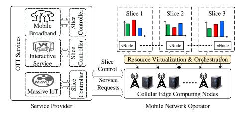
Figure 1.3: The network slicing in mobile edge computing network.
