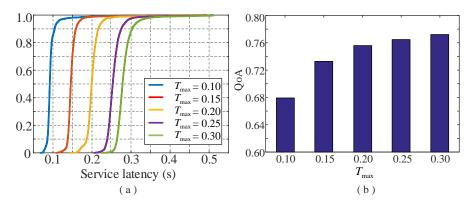
Figure 3.10: The performance of DARE with different  $T_{max}$ .
