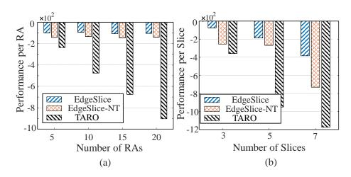
Figure 7.9: The scalability of EdgeSlice: (a) performance per RA vs. the number of RAs; (b) performance per slice vs. the number of slices.
