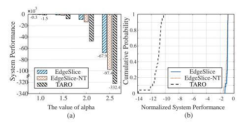
Figure 7.11: The compatibility of EdgeSlice: (a) system performance vs. the value of  $\alpha$ , (b) CDF of normalized system performance.
