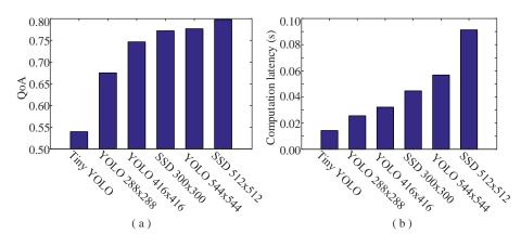
Figure 3.4: The QoA and latency v.s. the computation models.
