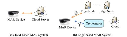
Figure 1.2: The cloud-based vs. edge-based MAR system.
