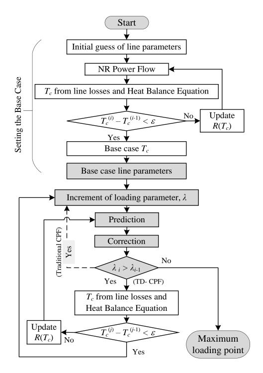
Figure 4.4: Temperature-Dependent Continuation Power Flow
