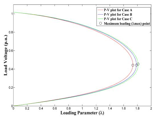
Figure 4.2: P-V plots for bus 2 for each case of the 4-bus system
