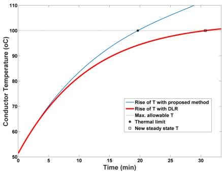
Figure 6.7: Line 1 conductor temperature – Case B
