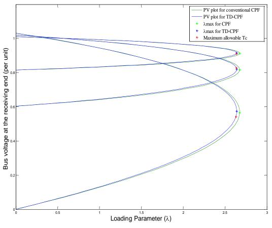
Figure 4.7: Conventional CPF and TD-CPF plots for the 3-segment line model (Cases 2 and 4)
