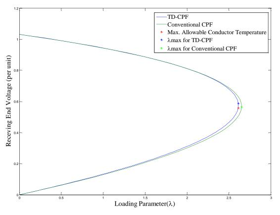
Figure 4.6: Conventional CPF and TD-CPF plots for the single-segment line model at weighted average conductor temperature (Cases 1 and 3)
