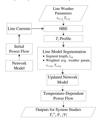
Figure 3.3: Integration of T-D line modeling with temperature-dependent PF
