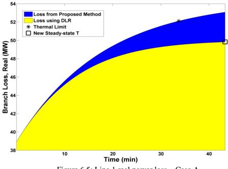
Figure 6.5: Line 1 real power loss – Case A
