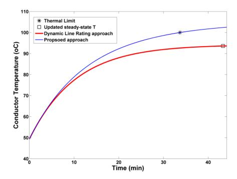
Figure 6.3: Line 1 conductor temperature – Case A
