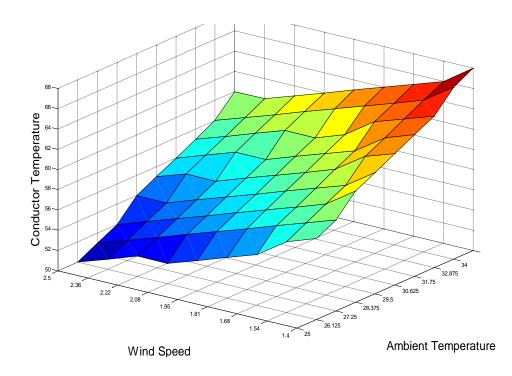
Figure 5.1: Conductor temperature as a function of ambient temperature and wind speed during the summer season
