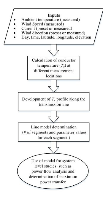
Figure A1: Process for multi-segment line modeling
