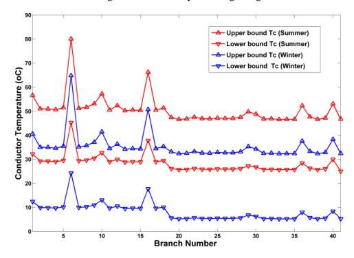
Figure 5.7: Conductor temperatures from proposed TD-PF
