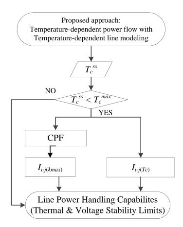
Figure 4.1: Power handling capability studies using temperature-dependent power flow
