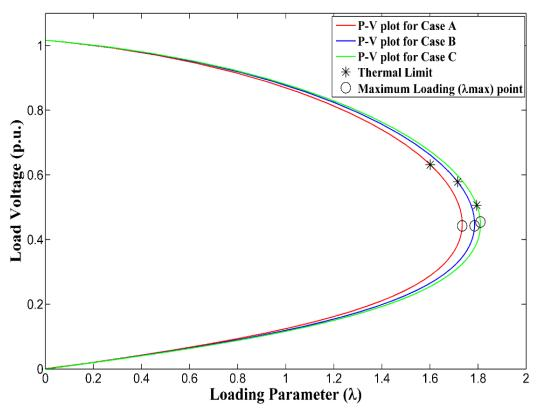
Figure 4.3: P-V plots with thermal limits
