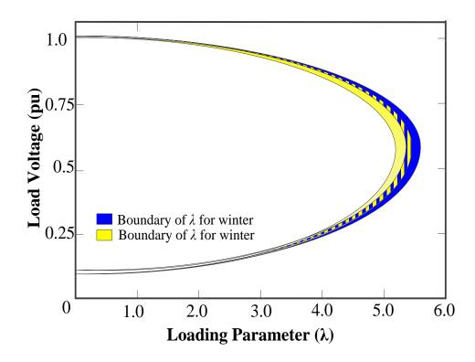
Figure 5.8: PV plot for 30-bus system
