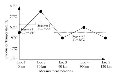
Figure 4.5:  $T_c$  profile and line model segmentation for case 2
