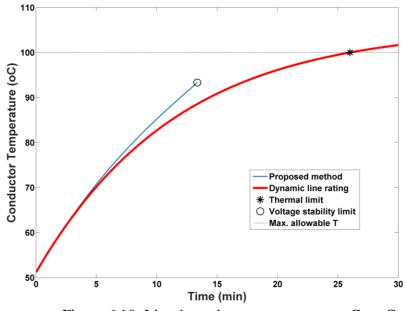
Figure 6.10: Line 1 conductor temperature – Case C
