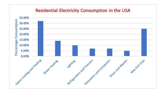
FIGURE 1.7: Residential electricity consumption in USA (2017)
