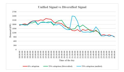
FIGURE 3.20: Unified vs diversified signals for EWHs
