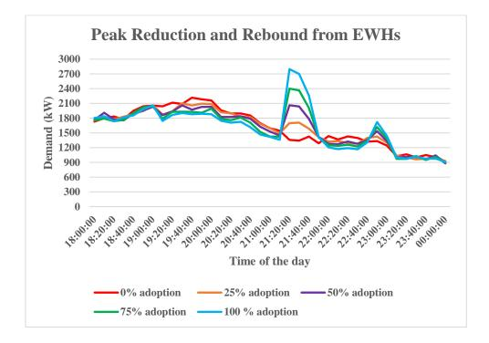
FIGURE 3.17: Peak reduction and rebound from water heaters
