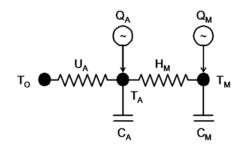
FIGURE 2.2: Equivalent thermal parameter model of a home in GridLAB-D
