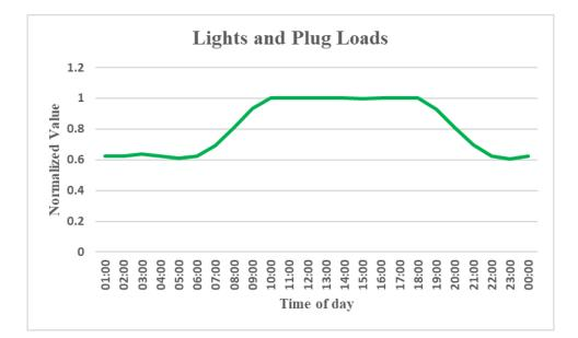
FIGURE 2.3: Demand profile for lights and plug loads
