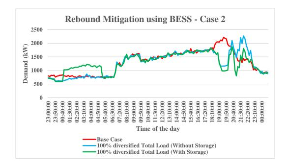
FIGURE 3.23: Rebound mitigation and load leveling for 100% DR and 25% BESS adoption scenario
