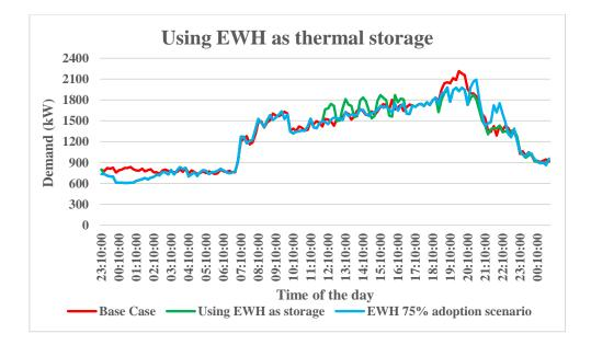
FIGURE 3.25: Using EWH as thermal energy storage
