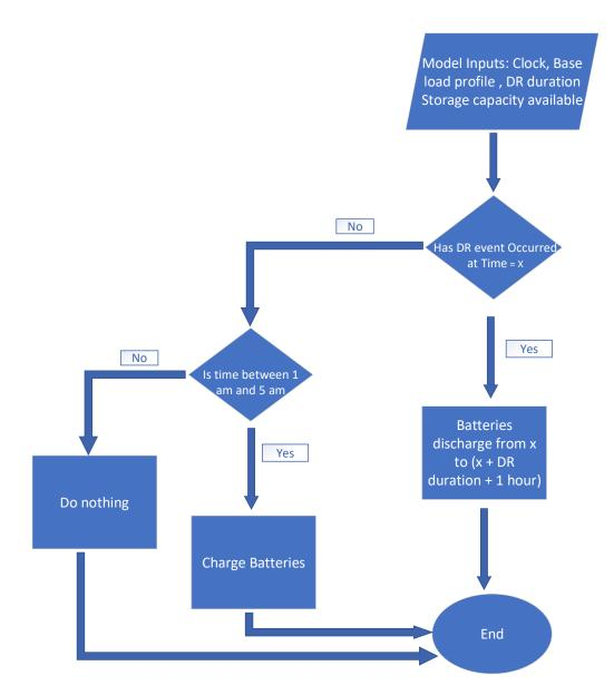
FIGURE 3.21: Battery scheduling algorithm for load leveling and DR mitigation
