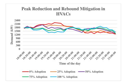
FIGURE 3.12: Peak reduction and rebound mitigation from HVACs
