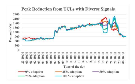
FIGURE 3.6: Rebound mitigation using diverse signals
