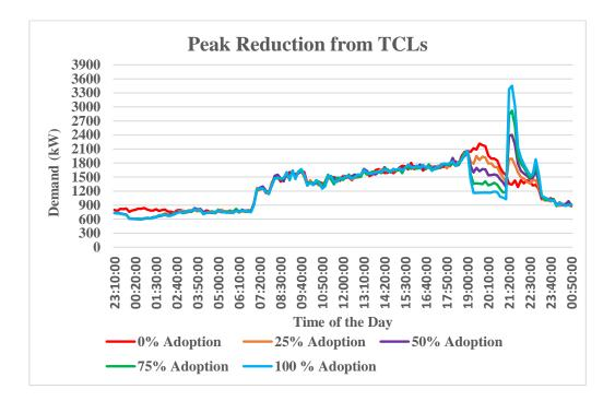
FIGURE 3.4: Peak reduction using TCLs
