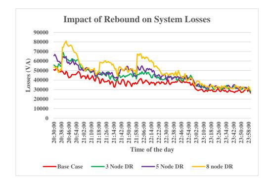
FIGURE 4.11: Impact of rebound on system losses
