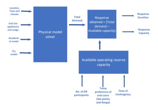
FIGURE 4.3: Operating reserves capacity architecture
