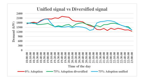
FIGURE 3.13: Unified vs Diversified signal for HVACs
