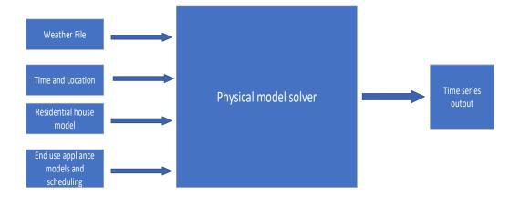
FIGURE 2.6: Architecture for building residential load models
