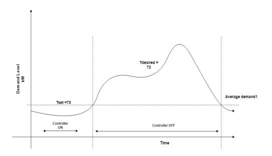
FIGURE 3.2: Graphical representation of pre-cooling mode
