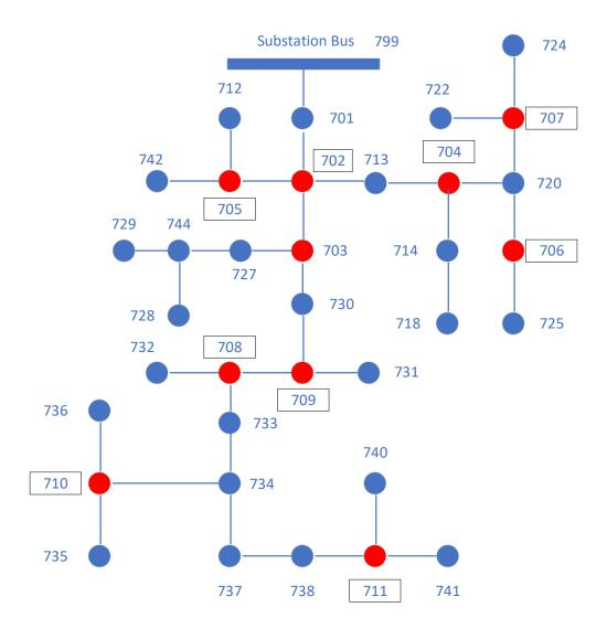
FIGURE 4.2: Nodes with provision to connect residential load
