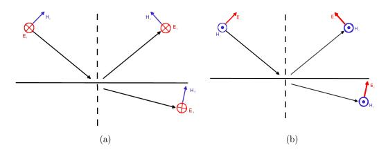
Figure 2.2: Two different operational modes of an incident wave; a) TE mode, b) TM mode
