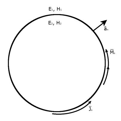
Figure 4.1: Surface Equivalence Principle for an arbitrary close surface
