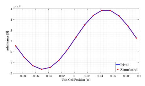
Figure 5.11: Admittance of the unit cell compared to the ideal admittance profile of the inside surface for the TM polarized wave steered at  $20^{\circ}$
