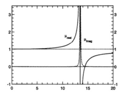
Figure 2.7: Permeability response of the geometry shown in Fig. 2.6 as frequency changes [4]
