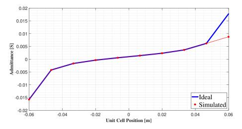
Figure 5.8: Admittance of the unit cell compared to the ideal admittance profile of the outside surface for the TE polarized wave steered at  $30^{\circ}$
