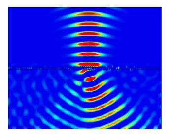
Figure 5.14: Near electric field response for the metasurface designed to steer  $30^{\circ}$  when excited with a TM Gaussian beam
