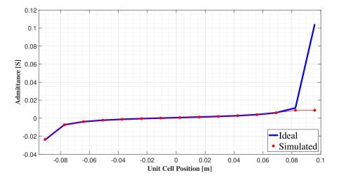
Figure 5.10: Admittance of the unit cell compared to the ideal admittance profile of the outside surface for the TM polarized wave steered at  $20^{\circ}$
