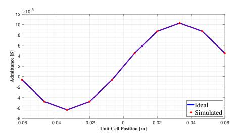
Figure 5.9: Admittance of the unit cell compared to the ideal admittance profile of the inside surface for the TE polarized wave steered at  $30^{\circ}$
