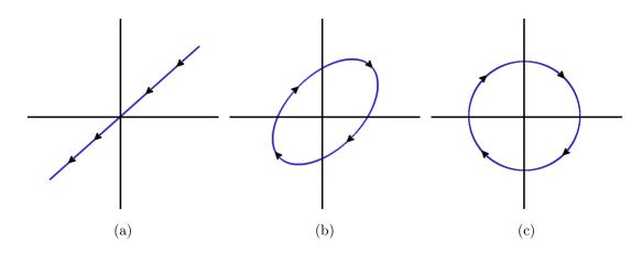
Figure 2.1: Three different polarization states for an electromagnetic wave; a) Linear polarization, b) Elliptical polarization, c) Circular polarization
