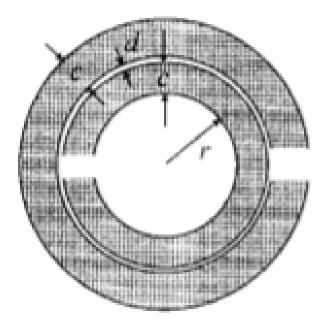
Figure 2.6: Periodic structure that shows a negative permeability at high frequencies [4]
