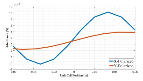
Figure 5.3: Ideal Admittance profiles for a 20° shift in the x-polarization and 30° in the y-polarization for  $Y_2$
