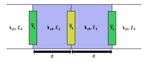
Figure 5.1: Approximate transmission line model for the metasurface
