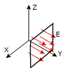
Figure 4.4: Orientation of a generic unit cell geometry for a y-polarized electric field of an incoming wave.
