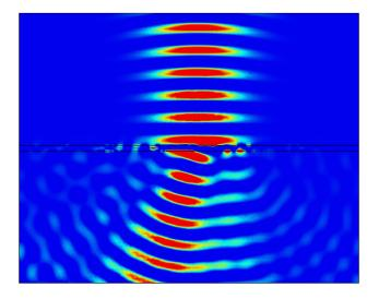
Figure 5.13: Near electric field response for the metasurface designed to steer  $20^{\circ}$  when excited with a TE Gaussian beam
