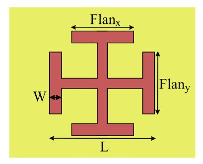
by the length of  $Flan_x$  and the admittance in the y-direction was effected by the length of  $Flan_y$ .
