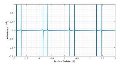
Figure 4.7: Surface Admittance across the surface of the metasurface.
