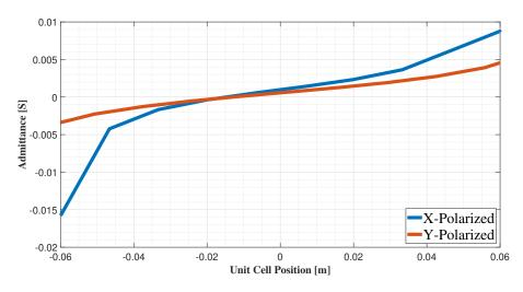
Figure 5.2: Ideal Admittance profiles for a 20° shift in the x-polarization and 30° in the y-polarization for  $Y_1$
