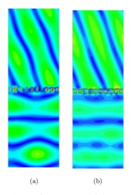
Figure 4.11: Near field radiation for the metasurfaces proposed in [6] for a) a TE polarized wave and b) a TM polarized wave
