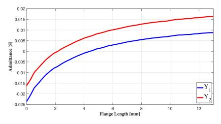
Figure 5.7: Admittance of the unit cell shown in Fig. 5.6 as the flange length is swept
