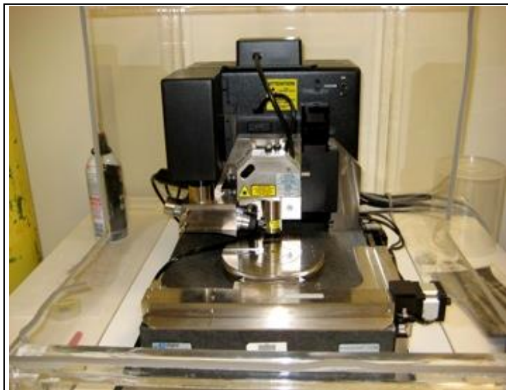
Figure 12: The Dimension 3100 SPM System with NanoScope IV Controller
