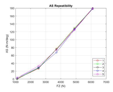
Figure 6.29: Aligning Stiffness Repeatability for Altimax 89
