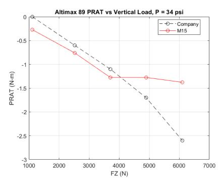
Figure 6.9: PRAT vs vertical load (Altimax 89)
