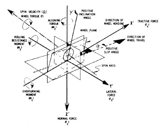
Figure 1.3: SAE Tire Axis System
