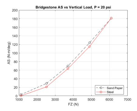
Figure 6.17: Aligning Stiffness (Sand paper vs Steel)
