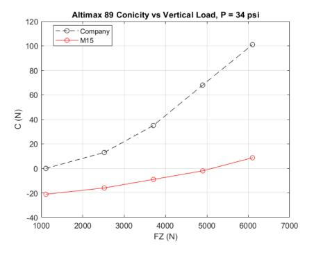
Figure 6.6: Conicity vs vertical load (Altimax 89)
