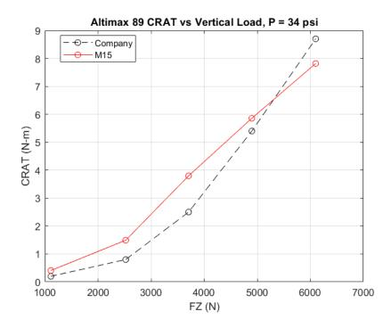
Figure 6.8: CRAT vs vertical load (Altimax 89)
