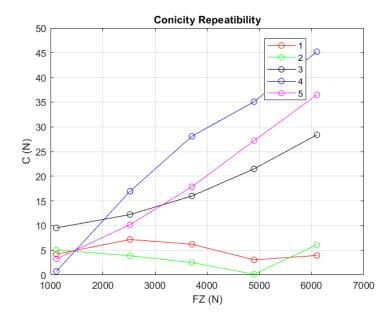
Figure 6.24: Conicity Repeatability for Altimax 89
