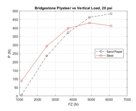
Figure 6.13: Ply Steer (Sand paper vs Steel)
