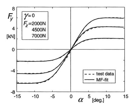
Figure 3.2: Magic Formula sample plot  $(F_y \text{ vs } SA)$
