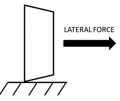
Figure 6.2: Conicity of tire
