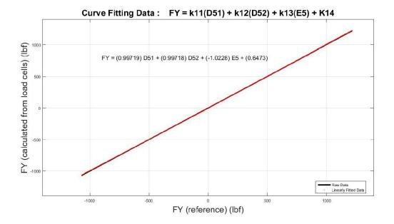
Figure 4.1:  $F_y$  equation after curve fitting
