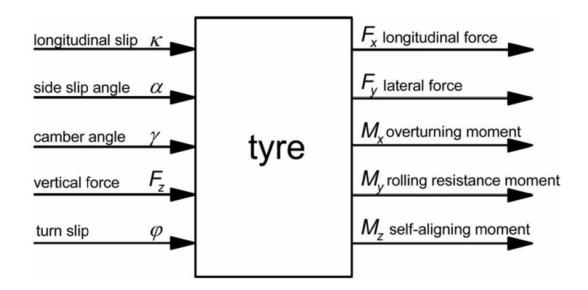
Figure 3.1: Tire inputs and outputs
