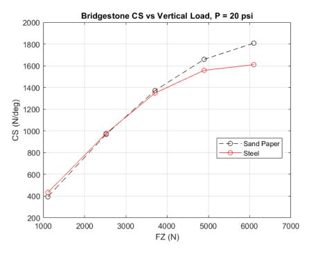
Figure 6.16: Cornering Stiffness (Sand paper vs Steel)
