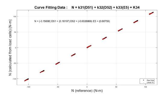
Figure 4.2:  $M_z$  equation after curve fitting
