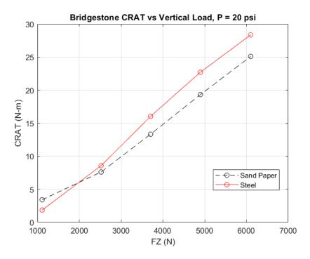
Figure 6.14: CRAT (Sand paper vs Steel)
