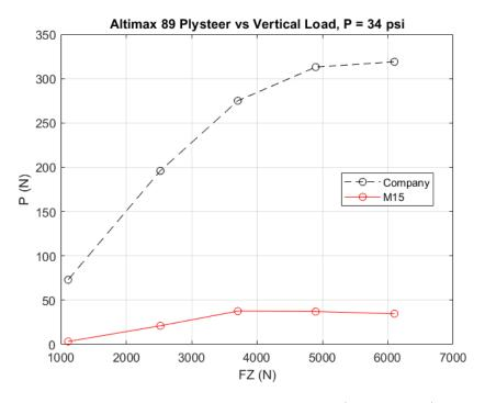
Figure 6.7: Ply Steer vs vertical load (Altimax 89)
