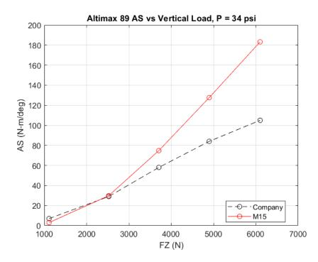
Figure 6.11: Aligning Stiffness vs vertical load (Altimax 89)
