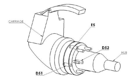
Figure 1.6: Load Cell Positions in the Carriage
