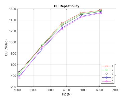
Figure 6.28: Cornering Stiffness Repeatability for Altimax 89
