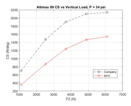
Figure 6.10: Cornering Stiffness vs vertical load (Altimax 89)
