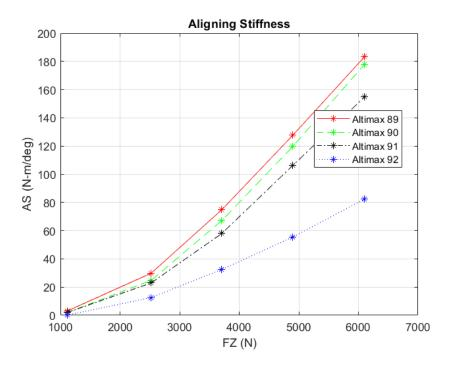
Figure 6.23: Aligning Stiffness for all Altimax tires
