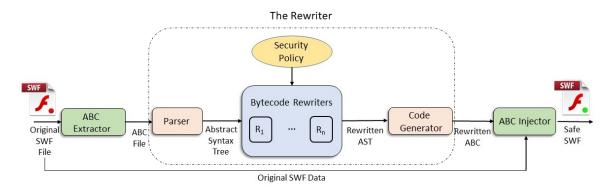
Figure 4.2: IRM Instrumentation as Bytecode Instructions [210]
