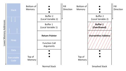
Figure 3.12: Structure of the call stack with buffer overflow vulnerability
