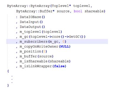
Figure 3.7: Implementation of the constructor function of ByteArray class
