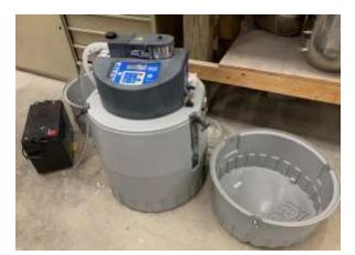
Figure 9: ISCO 6712 Sampler with 730 Flow Bubbler Module
