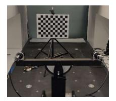
Fig. 6.6. Checkerboard used for calibration.
