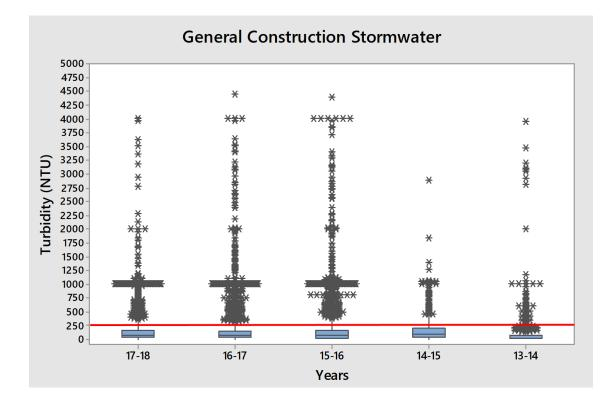
Figure 2 Box and whisker plot of turbidity values for general construction stormwater data
