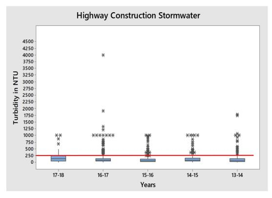
Figure 3 Box and whisker plot of turbidity values for Highway Construction Stormwater data
