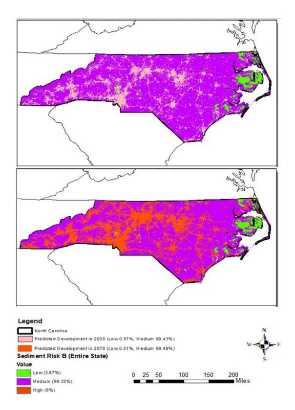
Figure 9 Sediment Risks for 1000 feet slope length and 2% slope angle with predicted development in 2030 and 2070
