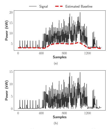
Figure 4.4: An example of (a) baseline estimation along with the (b) detrended signal. tion.
