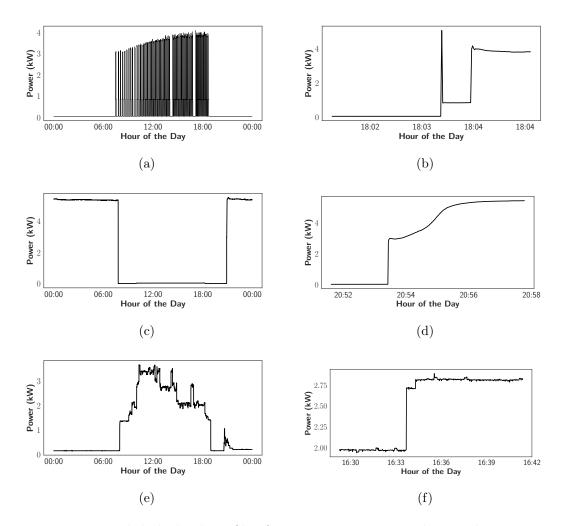
Figure 2.3: Typical daily load profiles for various circuits in the retail environment. (a) Air conditioner, (c) exterior lighting, and (e) interior lighting and Typical transient profiles for various circuits in the retail environment (b) Air conditioner, (d) exterior lighting, and (f) interior lighting.
