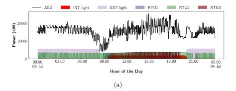
Figure 3.5: An example of aggregate power consumption, along with individual load constituents, for a typical weekday in a commercial building.
