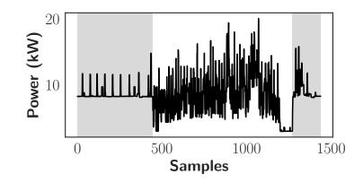
Figure 4.3: An example of the output of the change of mean detection algorithm, highlighted by the grey area.
