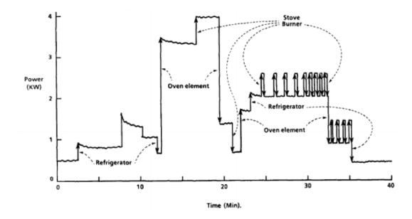
Figure 1.5: An example of the aggregate electricity signal explained by it's individual constituents [1].
