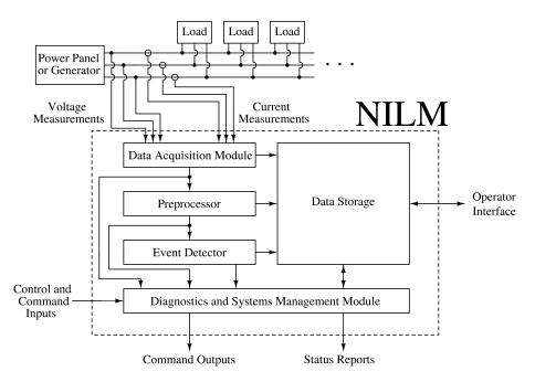
Figure 2.2: The fundamental signal flow path in a standalone NILM.
