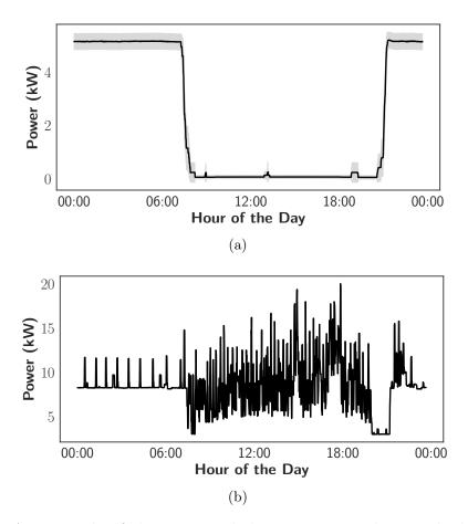
Figure 4.2: An example of the Exterior light uncertainty along with the aggregate power in a mid-size commercial building.
