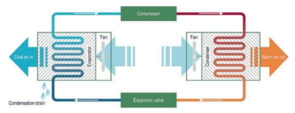
Figure 1.11: AC unit with a standard vapour compression refrigeration cycle.
