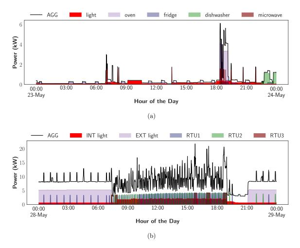
Figure 1.15: A comparison between the major individual constituents for a daily aggregate power consumption of (a) residential building and (b) commercial building.
