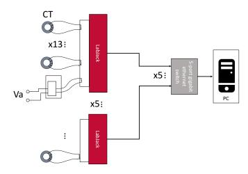
Figure 5.6: Basic hardware arrangement in the custom data-acquisition system.
