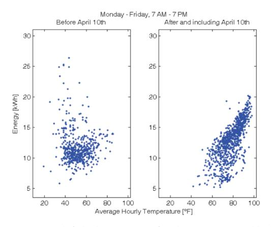
Figure 1.12: Example fault -detection process for a heat pump in a retail bank in Charlotte, North Carolina. Left shows a lack of correlation between outdoor air temperature and HVAC energy for HVAC unit with faulty compressor.
