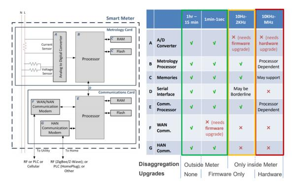
Figure 1.14: Typical arrangement for a utility-installed smart meter along with the respective constraints for different frequencies of metering [2].
