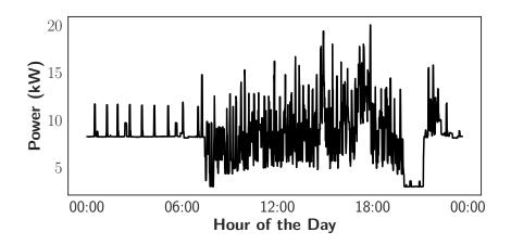
Figure 5.4: An example of a daily waveform in a commercial building.
