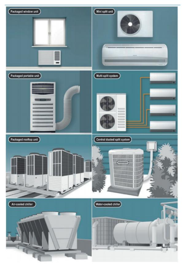
Figure 1.10: Common types of air-conditioning system.
