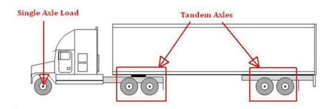
Figure 2.1: Tandem truck, single/tandem axles.
