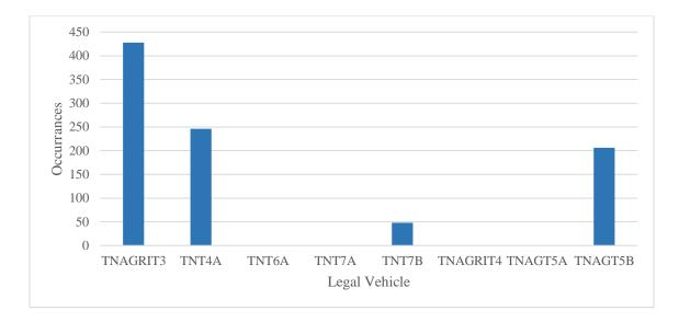
Figure 5.16: Posting vehicle frequency for all group 1 tandem trucks.
