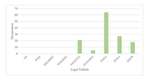
Figure 5.18: Posting vehicle frequency for all group 2 single unit vehicles.
