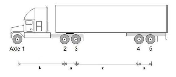
Figure 4.5: Truck axle spacing diagram with a/b/c distances.
