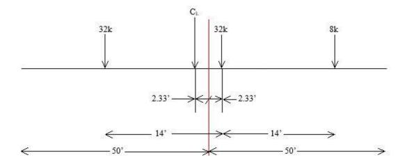
Figure 3.2: Line of action (in red) for HL-20 on a 100 ft. span bridge.
