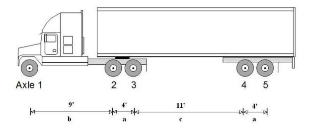
Figure 4: Truck Axle Spacing Diagram with a/b/c Distances.
