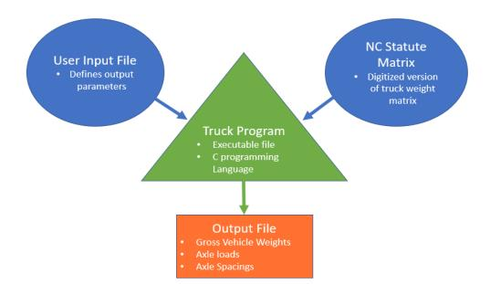
Figure 4.1: Legal truck generation program process visualization.
