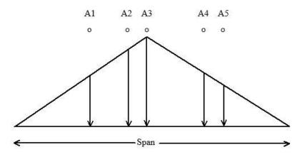
Figure 4.8: Graphic representation of influence line method of generating maximum bending moment.
