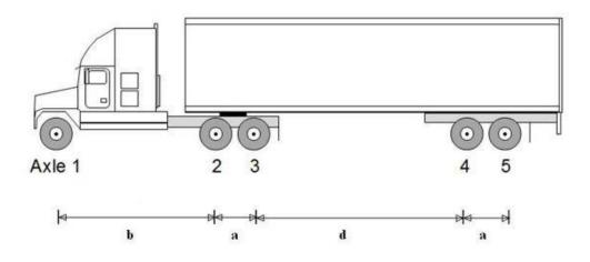
Figure 4.6: Truck axle spacing diagram with a/b/d distances.
