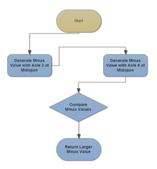
Figure 4.9: Maximum bending moment calculation logic diagram.
