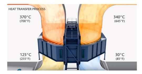
Figure 1.10: Heat Transfer Process in a Rotary Regenerative Air preheater (Temperature profile not pertaining to this study) [34]
