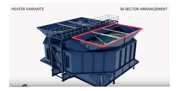
Figure 1.8: Bisector Rotary Regenerative Air preheater [34]
