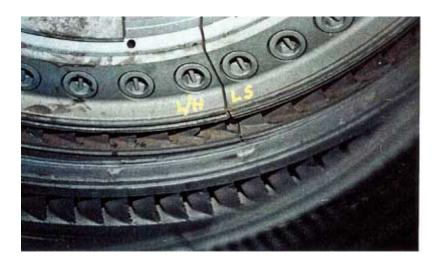
Figure 3.12: Nozzle Block Solid Particle Erosion (Courtesy: TG Advisers Inc.) [52, 53]
