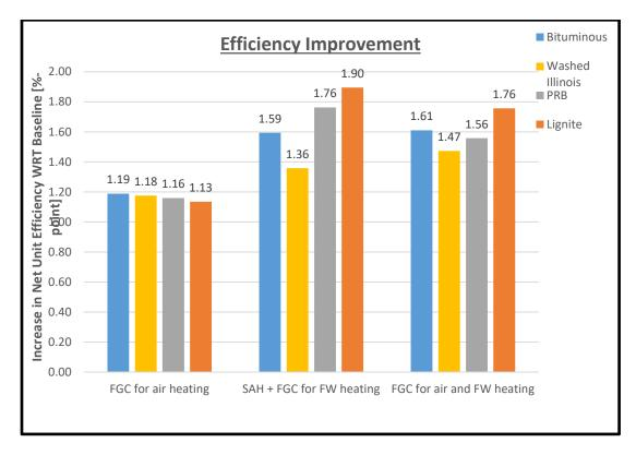
Figure 2.7: Increase in Net Unit Efficiency as a Function of Configuration and Coal Type
