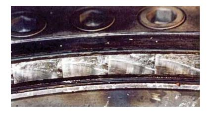
Figure 3.13: Vanes Solid Particle Erosion (Courtesy: TG Advisers Inc.) [52, 53]
