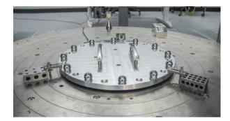
Figure 4.6. Upper plate clamped on the RT for stability test
