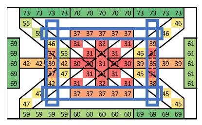
FIGURE 4.13: VHES miniature slab 7-day SR - standard reinforcement
