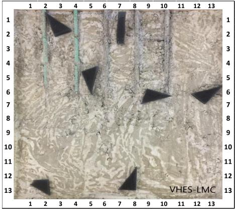
FIGURE 4.55: VHES-LMC mockup void locations
