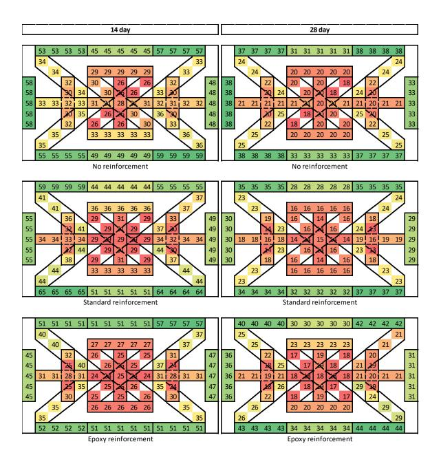
FIGURE C.4: 14 and 28 day VHES miniature slab data
