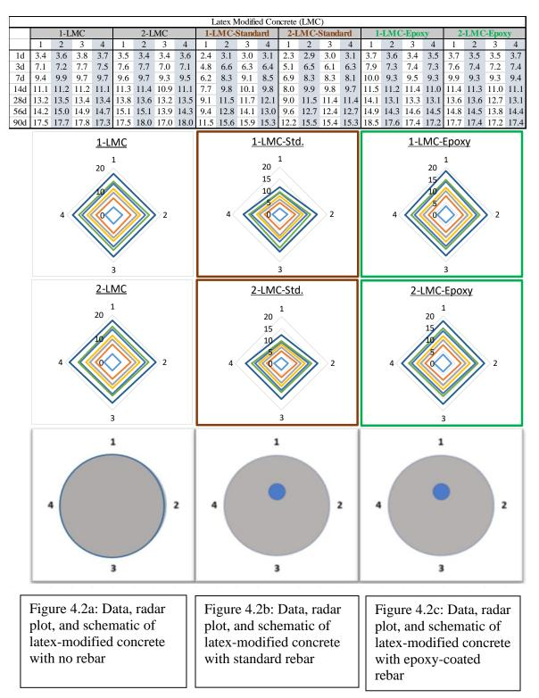
FIGURE 4.2: SR radar analysis for preliminary LMC cylinders
