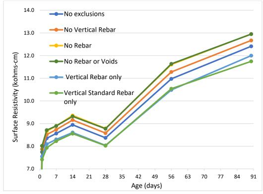
FIGURE 4.53: VHES mockup average of orientations with different exclusions
