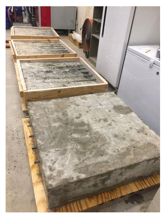
FIGURE 3.8: Control mockup and three overlay mockups pre-overlay
