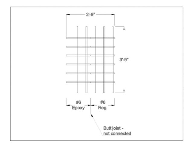
FIGURE 3.5: Typical bridge deck mockup steel reinforcement mat
