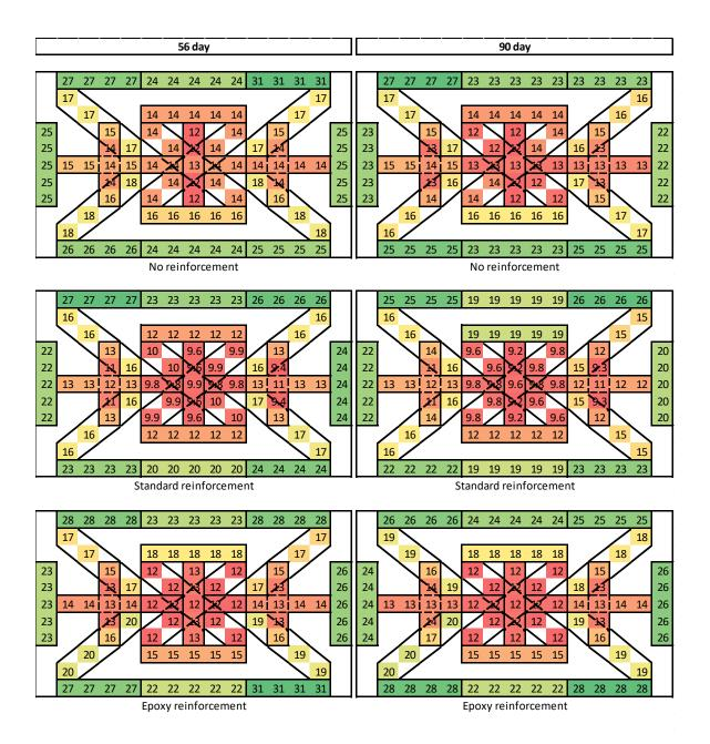
FIGURE C.5: 56 and 90 day VHES miniature slab data
