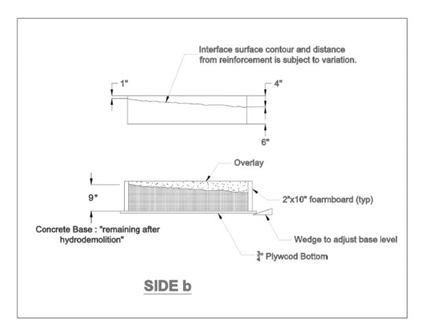
FIGURE 3.6: Typical bridge deck mockup section view
