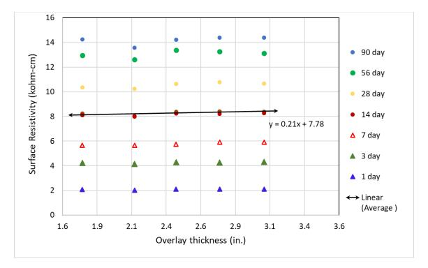
FIGURE 4.33: SR versus LMC overlay thickness
