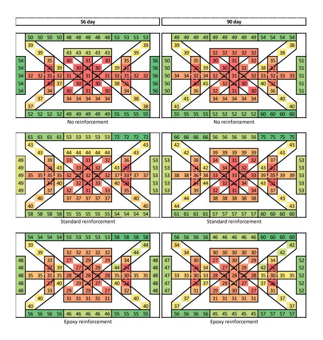
FIGURE C.9: 56 and 90 day VHES-LMC miniature slab data
