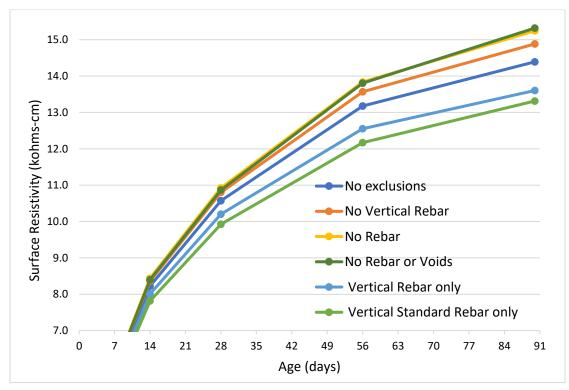
FIGURE 4.39: LMC mockup - SR average of orientations with different exclusions
