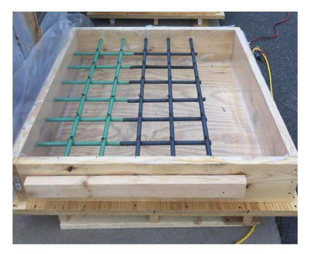
FIGURE 3.7: Typical bridge deck mockup form
