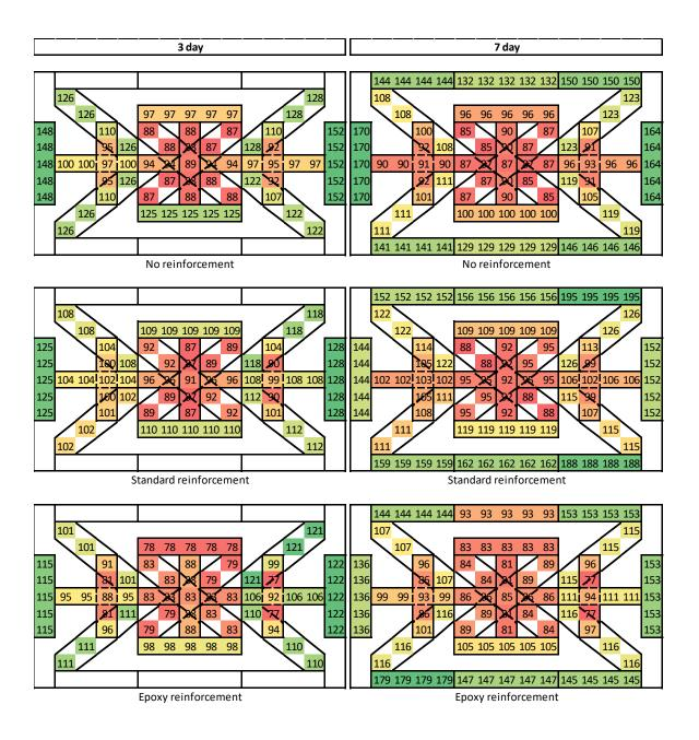
FIGURE C.7: 3 and 7 day VHES-LMC miniature slab data
