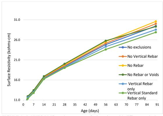
FIGURE 4.67: VHES-LMC mockup average of orientations with different exclusions
