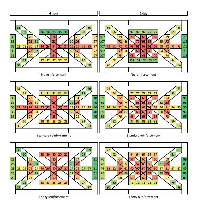
FIGURE C.6: 4 hour and 1 day VHES-LMC miniature slab data
