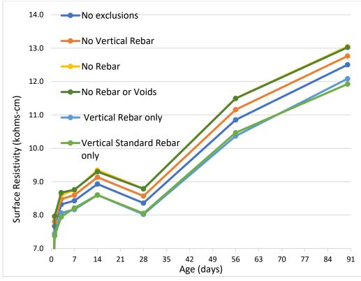
FIGURE 4.51: VHES mockup horizontal orientation with different exclusions
