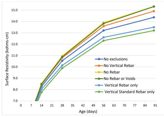
FIGURE 4.38: LMC mockup - SR vertical orientation with different exclusions
