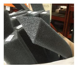
FIGURE 3.9: Polyether foam void material
