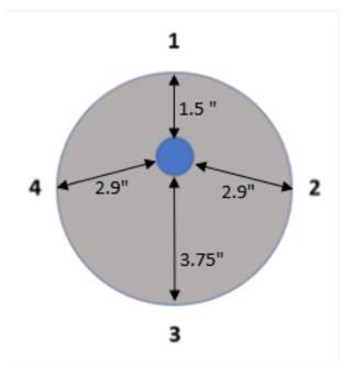
FIGURE 4.5: Cover depth of preliminary cylinders
