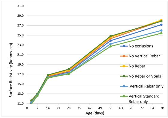
FIGURE 4.66: VHES-LMC mockup vertical orientation with different orientations
