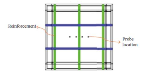
FIGURE 2.3: Probe configuration to reduce SR error
