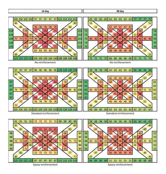
FIGURE C.8: 14 and 28 day VHES-LMC miniature slab data
