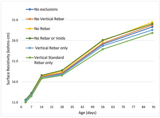
FIGURE 4.65: VHES-LMC mockup horizontal orientation with different exclusions
