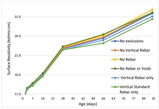
FIGURE 4.64: VHES-LMC mockup diagonal orientation with different exclusions
