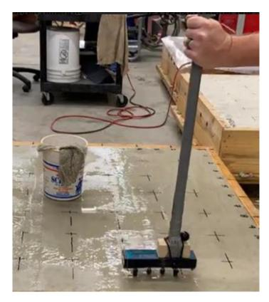
FIGURE 3.13: SR meter from standing position
