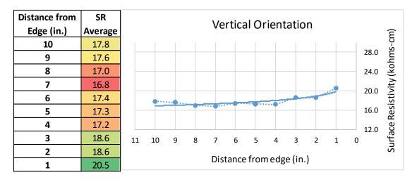
FIGURE 4.18: Graphical representation of SR edge effects
