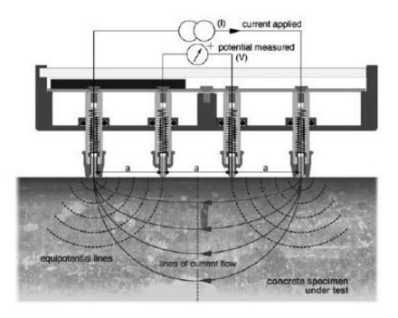
FIGURE 2.2: Proceq Resipod measurement principal (Proceq 2017)
