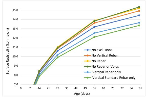
FIGURE 4.37: LMC mockup - SR horizontal orientation with different exclusions
