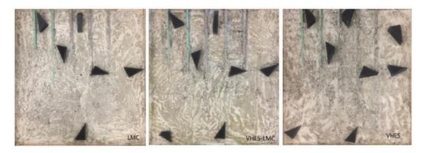
FIGURE 3.10: Mockup void placement - (a) LMC, (b) VHES-LMC, and (c) VHES
