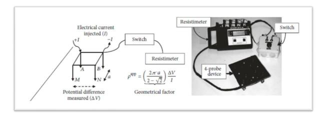
FIGURE 2.5: Four-probe square array principal (Lataste et al. 2003)
