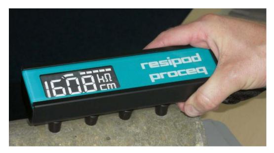
FIGURE 2.1: Proceq Resipod SR meter (Proceq 2017)
