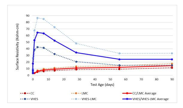
FIGURE 4.11: SR of preliminary 6 in. x 12 in. cylinders
