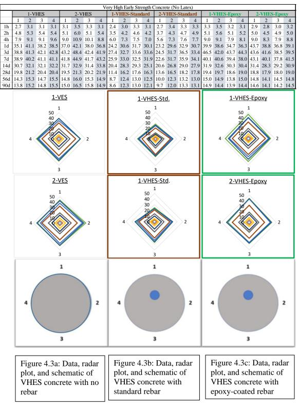
FIGURE 4.3: SR radar analysis for preliminary VHES cylinders
