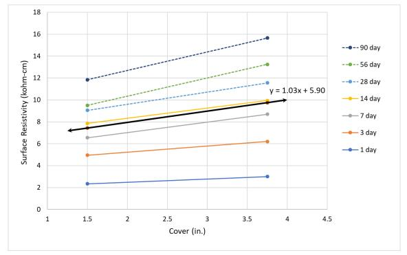
FIGURE 4.7: SR versus concrete cover at selected concrete ages - LMC mixture
