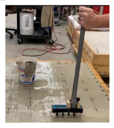
FIGURE 5.3: Measuring SR in the standing position
