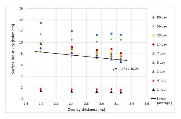
FIGURE 4.47: SR versus VHES overlay thickness
