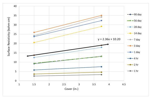
FIGURE 4.8: SR versus concrete cover at selected concrete ages - VHES Mixture
