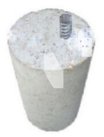
FIGURE 3.2: Typical 6 in. x 12 in. reinforced cylinder
