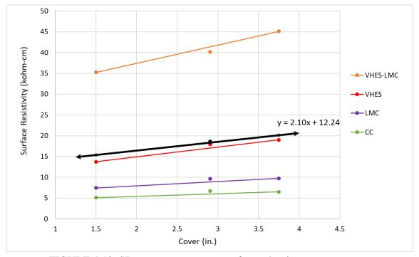
FIGURE 4.10: SR versus concrete cover for each mixture age average
