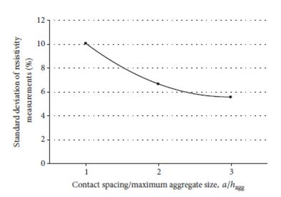
FIGURE 2.4: Effect of contact spacing on resistivity measurement
