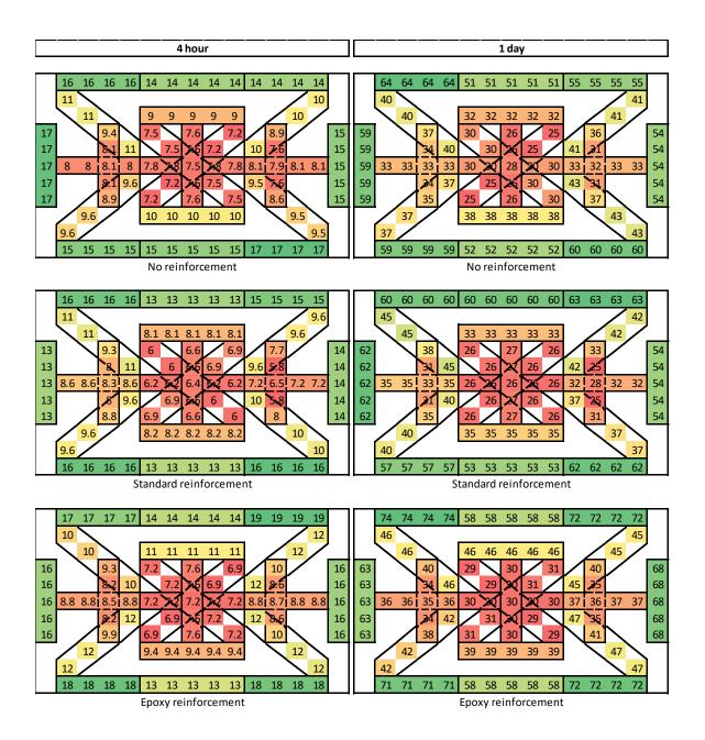
FIGURE C.2: 4 hour and 1 day VHES miniature slab data
