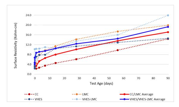
FIGURE 4.68: SR (kohm-cm) graph of CC ready-mix, LMC, VHES, and VHES-LMC 4
