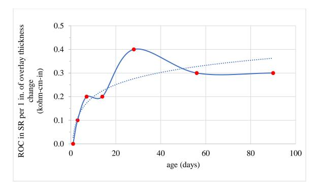
FIGURE 4.34: LMC rate of change per age (overlay thickness vs. SR)
