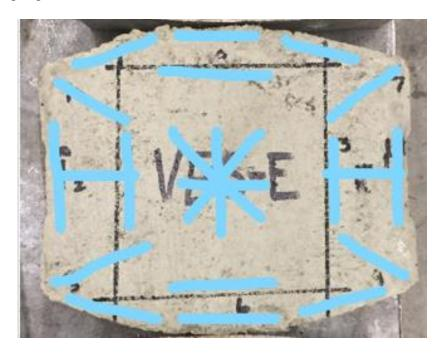
FIGURE 3.12: Typical miniature slab with location and orientation of rebar (shown in black) and test locations (shown in blue)
