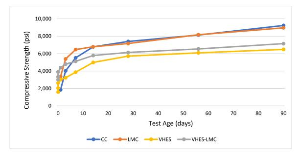
FIGURE 4.69: Compressive strength (psi) graph of CC ready-mix, LMC, VHES, and
