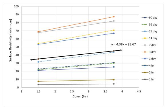
FIGURE 4.9: SR versus concrete cover pre age - VHES-LMC mixture
