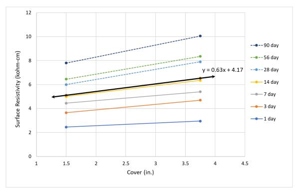
FIGURE 4.6: SR versus concrete cover at selected concrete ages - CC mixture
