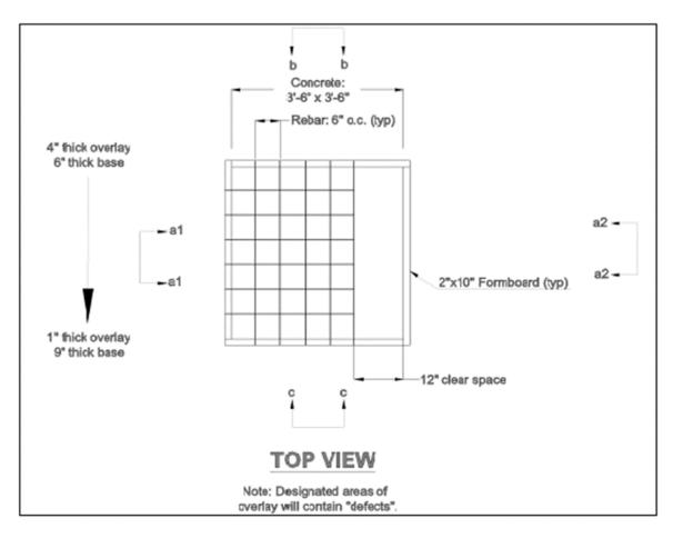
FIGURE 3.4: Plan view of typical bridge deck mockup schematic
