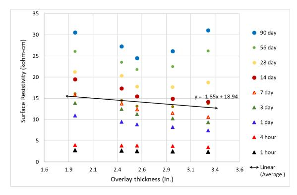
FIGURE 4.61: SR versus VHES-LMC overlay thickness
