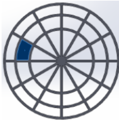
Figure 3.30: The figure is a cross sectional piece of the base design for the third generation samples. The waveguide is the truncated sector that is highlighted in blue.
