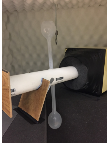
Figure 2.6: The physical experimental setup for the insertion loss experiment of two parallel HRs acting as side branches.
