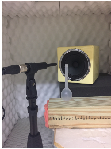
Figure 2.3: The physical setup for the single resonator experiment.
