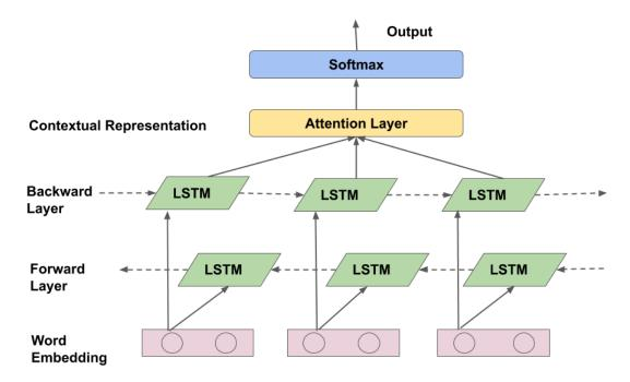
Figure 4.5: Enhanced LSTM for Natural Language Inference. Fig 4.5 is the baseline model to find agreement and disagreement in users interaction because it has been proved to be one of the best models for contradiction detection. This model uses Bi-LSTM to get the contextual representation and predicts the class of contradiction which in our cases are agreement, and disagreement.
