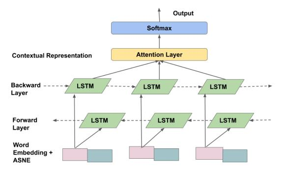
Figure 4.7: Enhanced LSTM for Natural Language Inference with ASNE.Fig 4.7 represents the architecture of another enhanced ESIM model. We tried to enhance it by adding ASNE along with glove embedding in the input layer.
