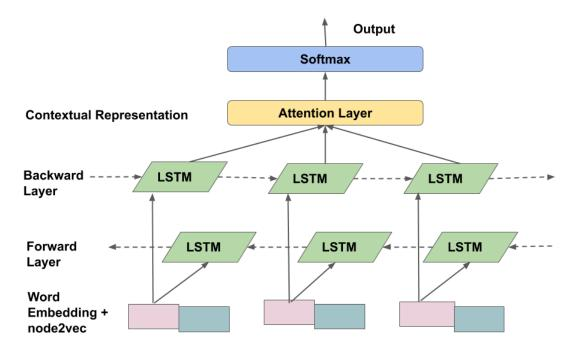
Figure 4.6: Enhanced LSTM for Natural Language Inference with node2vec. Fig 4.6 represents the architecture of the enhanced ESIM model. We tried to enhance it by adding node2vec along with glove embedding in the input layer.
