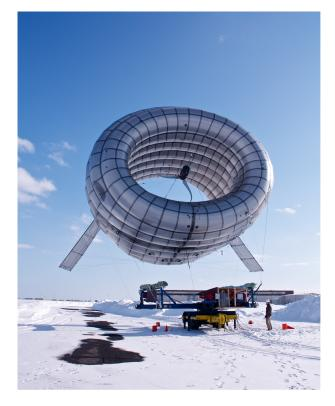
Figure 3: Full-scale prototype of Buoyant Airborne Turbine (BAT) during 2012 flight testing at Loring Air Force Base. [31]
