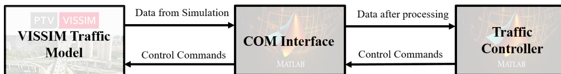
Figure 5.3: Data Transfer between Vissim-COM-Controller
