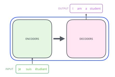
Figure 8.1: Basic Transformer Architecture used for Machine Translation [2]
