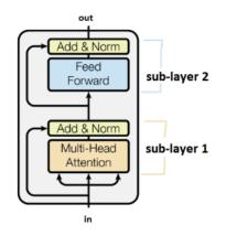
Figure 9.6: Transformer Encoder showing multi-head attention layer and the Feed Forward Neural Network
