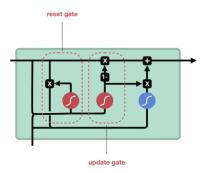
Figure 6.1: Gated Recurrent Units with Reset and Update Gate
