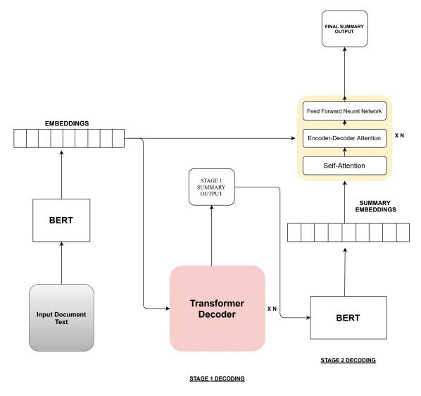
Figure 10.1: The novel BERT architecture with multi stage decoding
