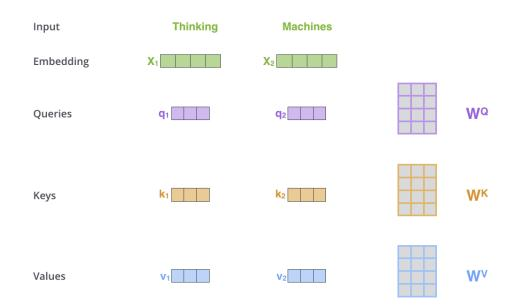
Figure 8.3: Multiplying x1 by the WQ weight matrix produces q1, the "query" vector associated with that word. We end up creating a "query", a "key", and a "value" projection of each word in the input sentence.
