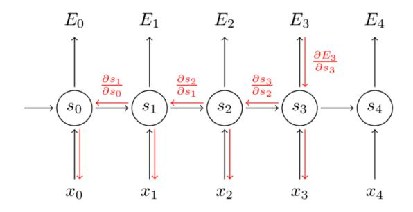
Figure 4.2: BPTT by summing up the gradients at each time step
