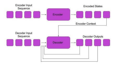
Figure 7.1: Sequence to Sequence Model - the encoder outputs a sequence of states. The decoder is a language model with an additional parameter for the last state of the encoder. [1]
