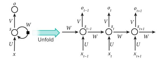
Figure 4.1: A recurrent neural network and the unfolding in time of the computation involved in its forward computation.
