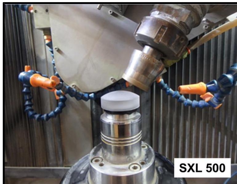
FIGURE 84: Grinding setup in SXL500 (the part is not silicon carbide in this Figure)
