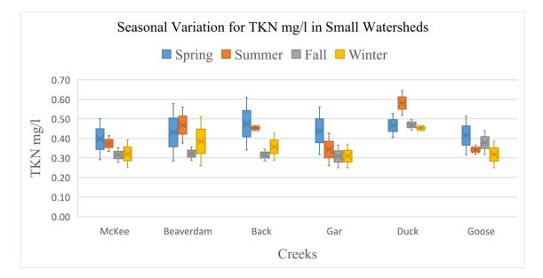
Figure 5: Variation in Total Kjeldahl Nitrogen mg/l across seasons during stormflow & base flow for Small Watersheds
