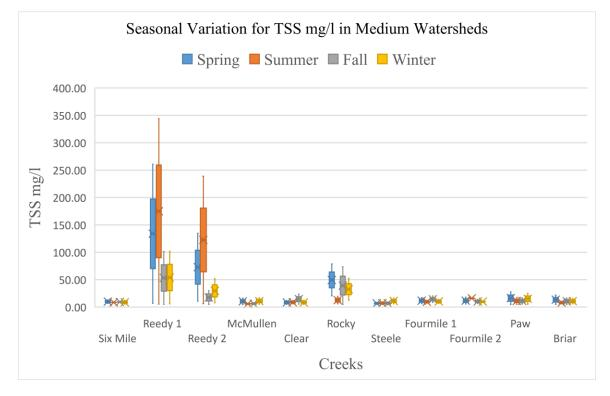
Figure 3: Variation in Total Suspended Solids mg/l across seasons during stormflow & base flow for Medium Watersheds
