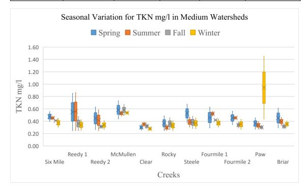
Figure 6: Variation in Total Kjeldahl Nitrogen mg/l across seasons during stormflow & base flow for Medium Watersheds
