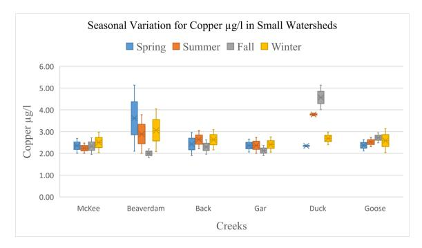
Figure 8: Variation in Copper  $\mu g/l$  across seasons during stormflow & base flow for Small Watersheds
