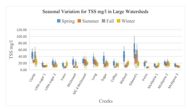
Figure 4: Variation in Total Suspended Solids mg/l across seasons during stormflow & base flow for Large Watersheds
