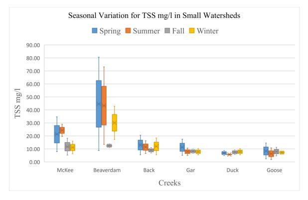
Figure 2: Variation in Total Suspended Solids mg/l across seasons during stormflow & base flow for Small Watersheds
