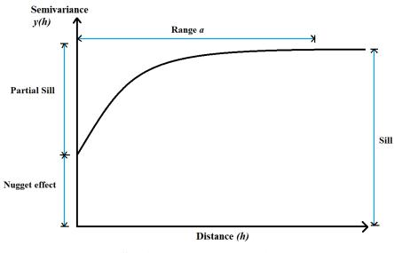
Figure 12 Semi-variogram plot (with components)
