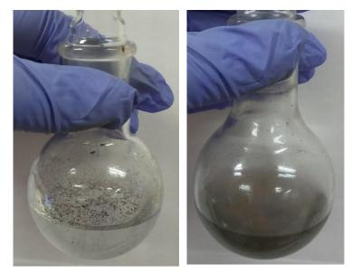
Figure S4.11: Different batches of controlled experiments in reflux (a) FGi in water (b) FGi and PEG in water under reflux for 3 days
