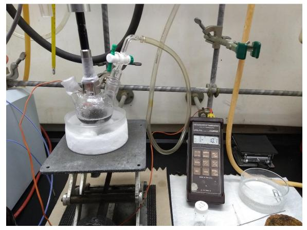
Figure S3.14: Schlenk apparatus with sonicator probe sealed and vessel under Ar(g) positive pressure
