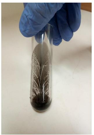
Figure S2.1: After centrifugation at 100,000 RCF (1 h), the reaction mixture deposits at the wall of the polycarbonate tubes
