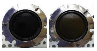
Figure 3.2: NanoResin membrane before any breakthrough experiments (left) and then after the 3<sup>rd</sup> breakthrough experiment (right). Yellow tinge on thin film (right) is from the NaFL adsorption.
