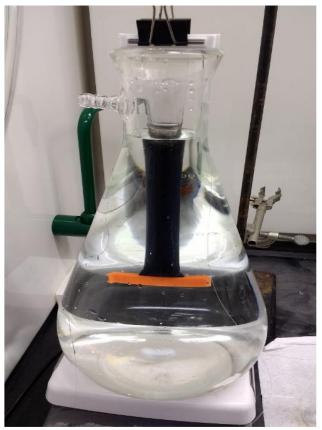
Figure S2.2: Brine removal from Aq-SNR dispersion. (A) Aq-SNR is the added in the form of dialyte and MilliQ is added as dialysate. The dialysate was replaced after every 2 h and then conductivity of dialysate was checked as a function of the number of iterations. This confirms maximal removal of brine (<1  $\mu$ S/cm).
