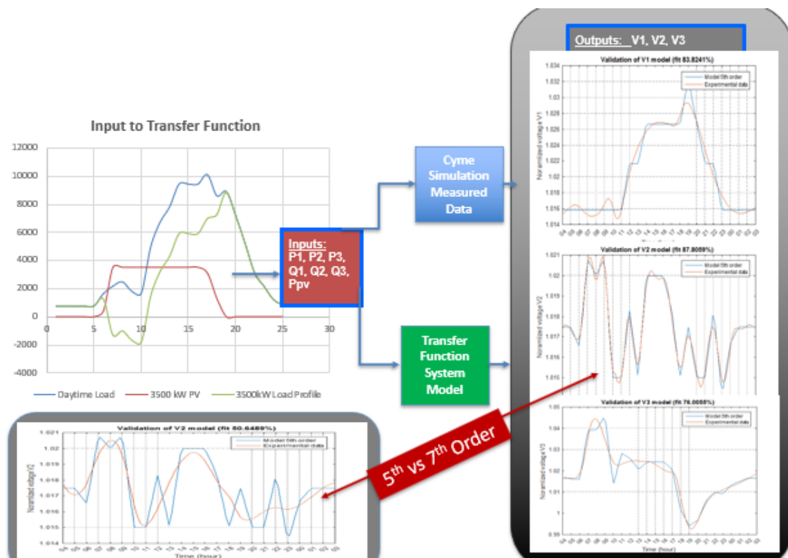
Figure 6.11: MIMO Model Comparison - Power Flow Simulation vs. Transfer Function Model
