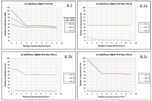
FIGURE 43: Number of rejections out of 1000 arrivals for 12 veh/hour arrival rate with higher first tier vehicle ratio vs number of pumps shared in tiers 1 (PS1) and 2.
