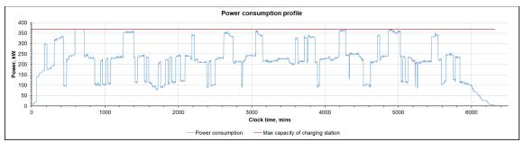
FIGURE 53: Power consumption profile for arrival rate of 10 veh/hour with BAR and
