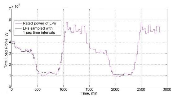
FIGURE 25: Total load profiles (TLPs) calculated for two scenarios: rated power of LPs and LPs sampled with 1 sec time intervals.
