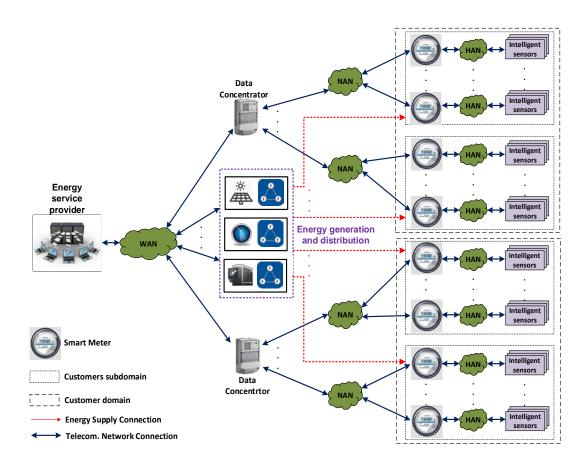
FIGURE 12: General example of telecommunication network supporting advanced metering infrastructure of SGs. Data from each customer domain is obtained through corresponding data concentrators and NANs, which consist from several HANs that are monitored by smart meters. WAN controls energy generation and distribution for the whole grid.
