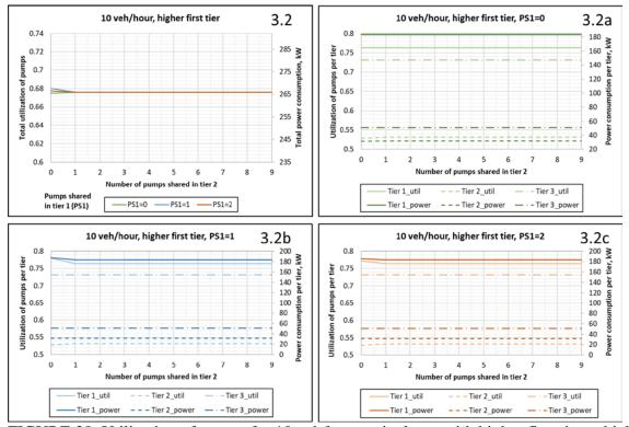
FIGURE 38: Utilization of pumps for 10 veh/hour arrival rate with higher first tier vehicle ratio vs number of pumps shared in tiers 1 (PS1) and 2.
