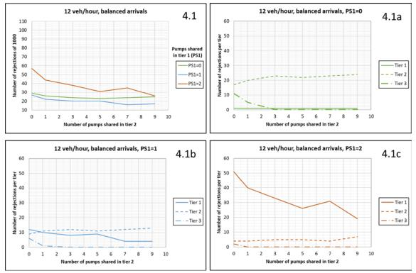
FIGURE 39: Number of rejections out of 1000 arrivals for 12 veh/hour arrival rate with balanced vehicle ratio vs number of pumps shared in tiers 1 (PS1) and 2.
