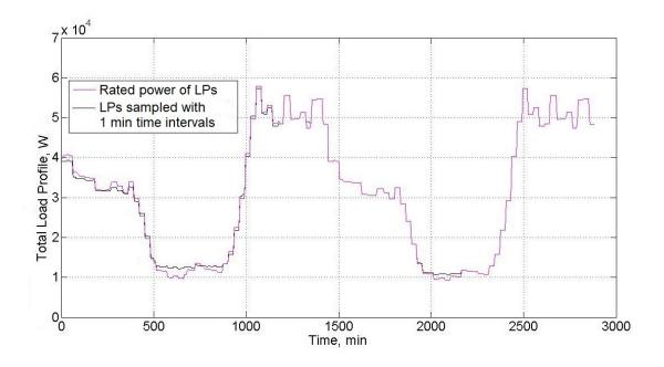
FIGURE 24: Total load profiles (TLPs) calculated for two scenarios: rated power of LPs and LPs sampled with 1 min time intervals.
