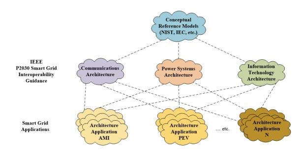
FIGURE 10: Scope of IEEE 2030 standardization process.
