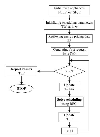
FIGURE 22: Flow chart of simulation implementation for dynamic load scheduling.
