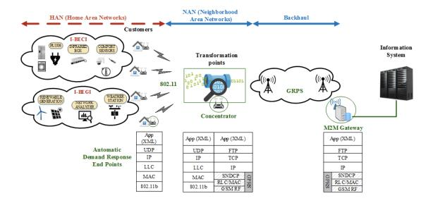
FIGURE 17: Mapping of the proposed M2M communications architecture onto the power distribution infrastructure.
