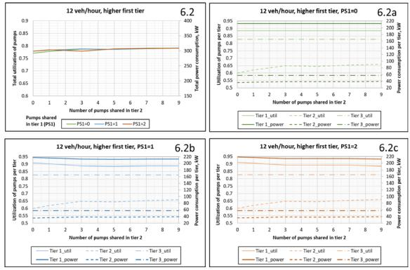
FIGURE 44: Utilization of pumps for 12 veh/hour arrival rate with higher first tier vehicle ratio vs number of pumps shared in tiers 1 (PS1) and 2.
