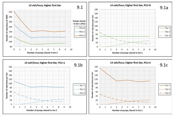
FIGURE 49: Number of rejections out of 1000 arrivals for 14 veh/hour arrival rate with higher first tier vehicle ratio vs number of pumps shared in tiers 1 (PS1) and 2.
