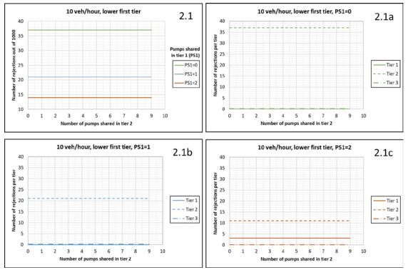
FIGURE 35: Number of rejections out of 1000 arrivals for 10 veh/hour arrival rate with lower first tier vehicle ratio vs number of pumps shared in tiers 1 (PS1) and 2.
