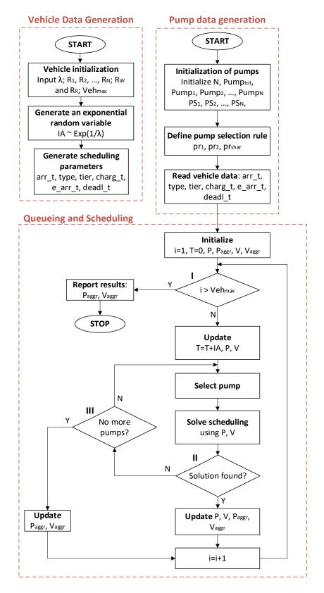
FIGURE 31: Flow chart of a simulation implementation of the online scheduling procedure
