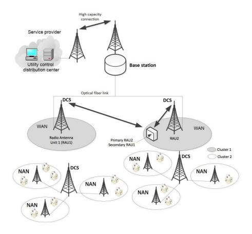
FIGURE 21: A part of SG telecommunication architecture based on the RoF technology with a two-tier hierarchical structure. The residential domain of SG is considered [139].
