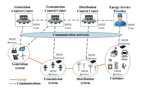
FIGURE 16: Mapping of the proposed M2M communications architecture onto the European Telecommunications Standards Institute (ETSI) M2M architecture applied to the Smart Grid.
