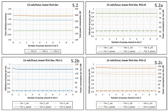
FIGURE 42: Utilization of pumps for 12 veh/hour arrival rate with lower first tier vehicle ratio vs number of pumps shared in tiers 1 (PS1) and 2.
