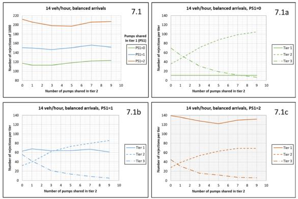
FIGURE 45: Number of rejections out of 1000 arrivals for 14 veh/hour arrival rate with balanced vehicle ratio vs number of pumps shared in tiers 1 (PS1) and 2.
