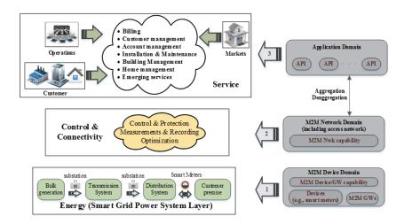
FIGURE 14: The structure of machine-to-machine (M2M) network for smart grids according to the European Telecommunications Standards Institute (ETSI). M2M domains are mapped onto the smart grid main layers.
