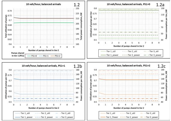
FIGURE 34: Utilization of pumps for 10 veh/hour arrival rate with balanced vehicle ratio vs number of pumps shared in tiers 1 (PS1) and 2.
