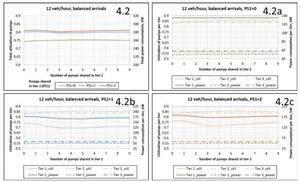
FIGURE 40: Utilization of pumps for 12 veh/hour arrival rate with balanced vehicle ratio vs number of pumps shared in tiers 1 (PS1) and 2.
