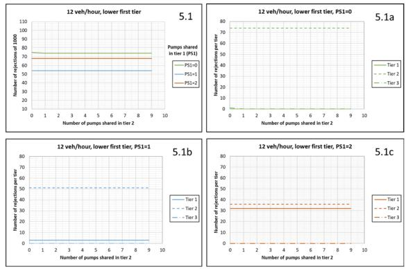
FIGURE 41: Number of rejections out of 1000 arrivals for 12 veh/hour arrival rate with lower first tier vehicle ratio vs number of pumps shared in tiers 1 (PS1) and 2.
