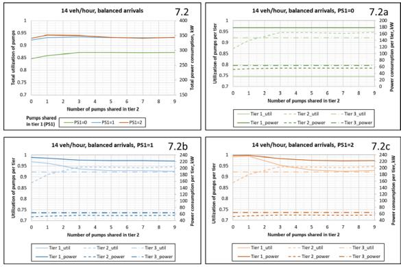
FIGURE 46: Utilization of pumps for 14 veh/hour arrival rate with balanced vehicle ratio vs number of pumps shared in tiers 1 (PS1) and 2.
