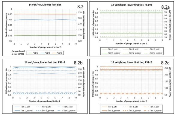
FIGURE 48: Utilization of pumps for 14 veh/hour arrival rate with lower first tier vehicle ratio vs number of pumps shared in tiers 1 (PS1) and 2.
