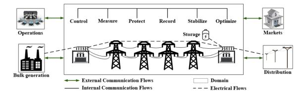
FIGURE 8: General architecture of the transmission domain.
