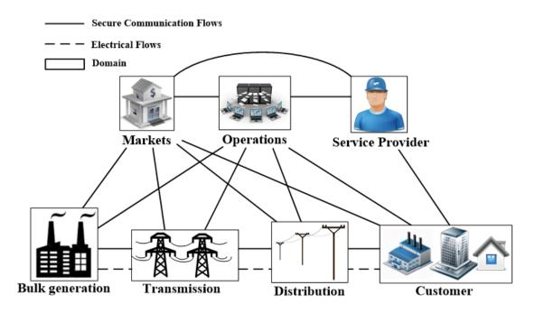
FIGURE 2: NIST Smart Grid Conceptual Model.
