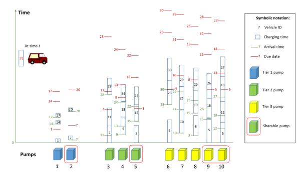
FIGURE 30: An example of optimal scheduling procedure scenario represented as a snapshot at the time of new vehicle arrival. Sharable pumps in each tier are framed in red.
