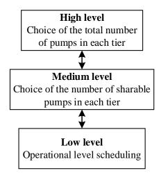
FIGURE 29: Main levels of decision-making hierarchy in an autonomous charging station.
