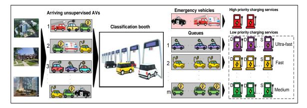
FIGURE 27: Traffic flow within an autonomous charging station. Designated (D) and sharable (S) pumps are considered [29].
