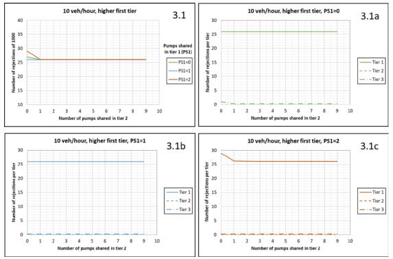
FIGURE 37: Number of rejections out of 1000 arrivals for 10 veh/hour arrival rate with higher first tier vehicle ratio vs number of pumps shared in tiers 1 (PS1) and 2.
