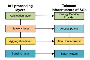
FIGURE 18: A relation between IoT processing layers and telecom infrastructure of SGs. Sensing, aggregation, network, and application layers are mapped on corresponding nodes of telecom infrastructure of SGs [41].
