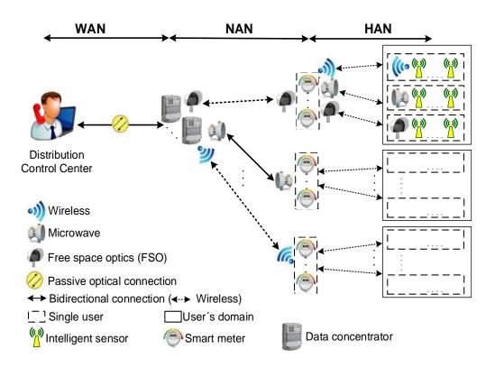
FIGURE 19: Schematic topology of a hybrid passive optical network (HPON) for an advanced metering infrastructure (AMI) of SG telecom network. HPON is implemented as a backbone network. Wireless, microwave, and free space optics technologies are considered for distribution and access networks.
