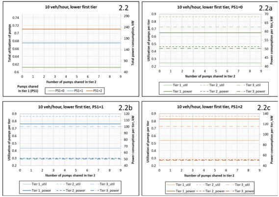
FIGURE 36: Utilization of pumps for 10 veh/hour arrival rate with lower first tier vehicle ratio vs number of pumps shared in tiers 1 (PS1) and 2.
