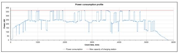
FIGURE 54: Power consumption profile for arrival rate of 12 veh/hour with BAR and charging station's design with non-sharable pumps only.
