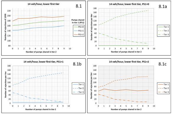
FIGURE 47: Number of rejections out of 1000 arrivals for 14 veh/hour arrival rate with lower first tier vehicle ratio vs number of pumps shared in tiers 1 (PS1) and 2.
