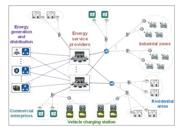
FIGURE 26: typical structure of energy distribution within smart grids.
