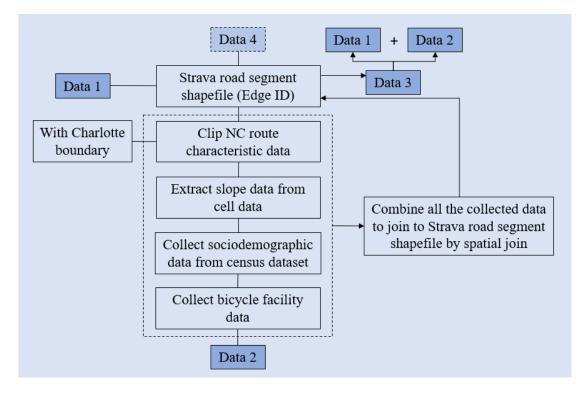
Figure 5.2: Data Processing in ArcGIS
