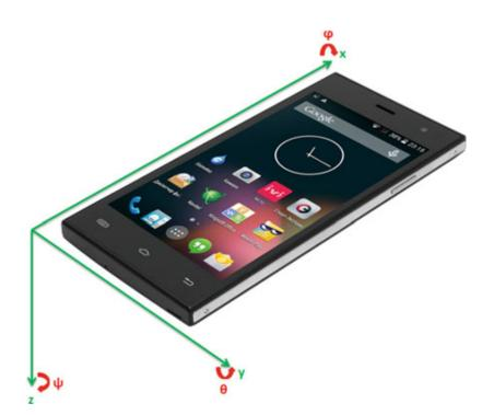
Figure A.35: The coordinate system of smartphones and corresponding orientation angles
