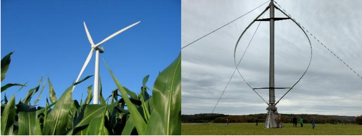
FIGURE 7- A Typical Horizontal Axis Wind Turbine (left) [19] and a Darrieus Type Vertical Axis Wind Turbine (right) [20]
