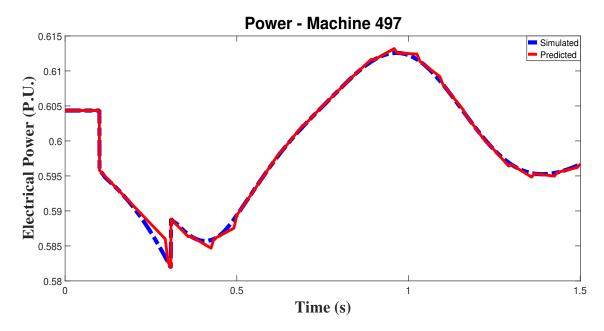
Figure 4.26: Actual and predicted output power of G497 that has the minimum error - Fault on bus 71 - 500 bus system.
