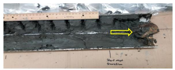
(Figure 4.2) Remnant of sediment catcher applied to prevent sample loss at yellow arrow.
