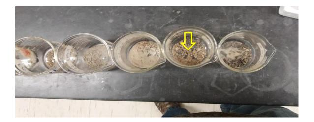
(Figure 1.1). Subsamples from core FM1. A fine layer of silt was found preserved between the sharp contact of the sand lens and marsh facies in the younger storm layer. The yellow arrow indicates the sample containing the silt layer.
