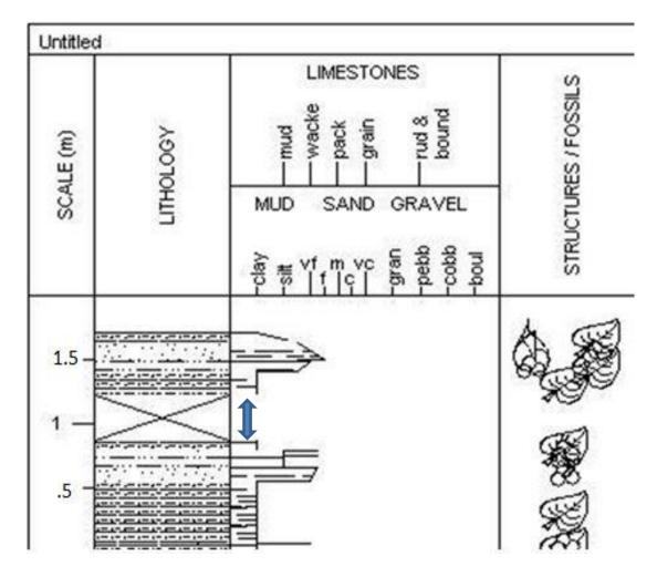
(Figure 5.13) FM8 displays fair sediment recovery with several intervals of clay, silt and sand along with marsh facies. Slumping in the middle has left 36-cm empty at 48-cm in depth to 84-cm (blue arrow). The sediment intervals of sand, silt, clay, and marsh mud is likely due to tidal channel sequences caused by meandering marsh creeks.
