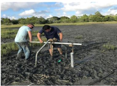
(Figure 4.1-B) Lance Zurawski and Steven Ortiz using the pry-and-lever system to remove a vibracore.
