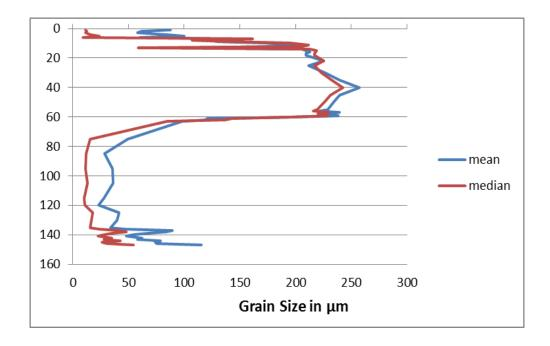
(Figure 5.15) FM1 mean and median changes in grain-size down core. Note the clear rise in grain size for the older storm layer in the interval between 142 and 148-cm.
