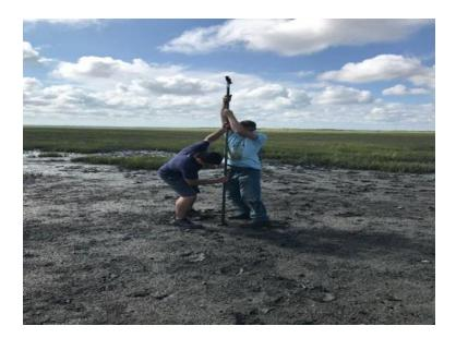
(Figure 4.1-A) Gauge auger probing for sand lenses.
