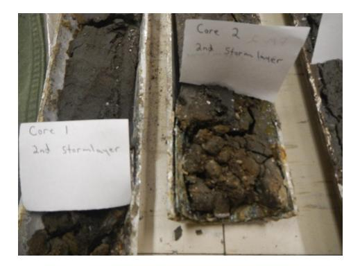
(Figure 5.16) Pedogenesis developing within the older storm layer containing clay and sand. The development of peds indicates the weathering processes responsible for soil development. Textural differences created by the storm layer, the presence of clay and silt, and the organic content together give the appearance of a soil horizon.
