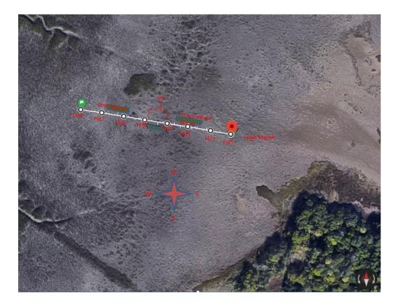
Figure 3.5. Google Earth aerial photo image of North Folly Island with coring site transect of 5 meter intervals marked to 40 meters in length.
