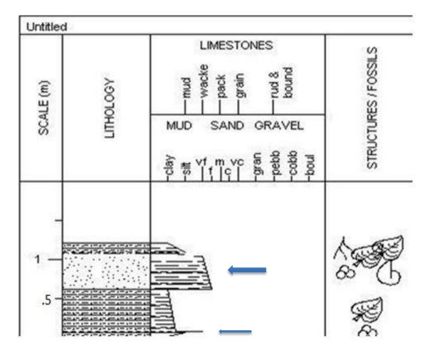
(Figure 5.12) FM7 contains a younger sand lens the same width as FM6. A smaller portion of the older storm layer is evident by offshore foraminiferal assemblages only. The lower layer is texturally unrecognizable from the marsh facies. Storm layers are located at the blue arrows.
