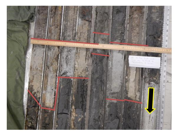
Figure 5.5. Moving from left to right FM1, FM2, FM3, FM4, FM5, FM6, FM7, and FM8. Continuous sand lenses appear to thin in the middle and thicken at the ends of the transect. Red lines depict the upper and lower contacts of the upper sand lens. Arrow at FM8 points to the direction the sand lens is found due to slumping of the sediment.
