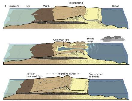
(Figure 3.2). The three-step process of barrier island rollover. Image from Warner College of Natural Resources.
