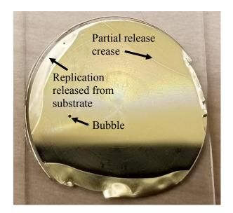
Figure 3.10 Replicated flat with 50nm of Gold
