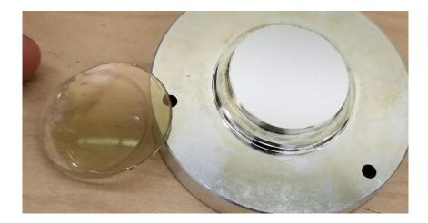
Figure 3.11 Aluminum flat sputtered with 25nm of Gold
