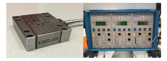
Figure 3.1 Kistler 3-axis dynamometer 9256C1 (left) and the charge amplifier (right)
