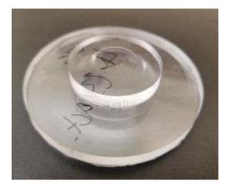
Figure 4.11 PMMA 'top hat' stamper with 25 µm deep cylindrical recess.
