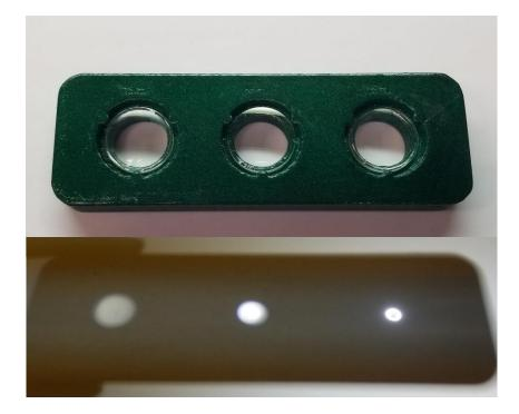
Figure 2.8 Three optic demonstrator with increased focal length/decreased power (left) original lens substrate (center) and decreased focal length/increased power (right)
