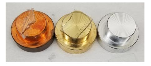
Figure 2.1 Copper, brass, and aluminum stampers with sinewave
