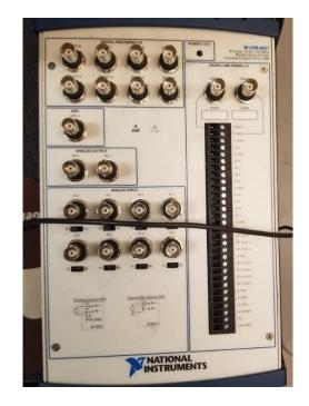
Figure 3.2 National Instruments USB-6251 DAQ board
