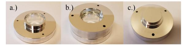
Figure 2.9 New replication system using spacer ring comprising substrate holder a.) spacer ring b.) and stamper c.)
