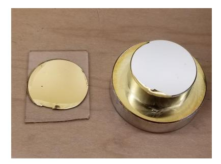
Figure 3.9 Aluminum flat sputtered with 50nm of gold
