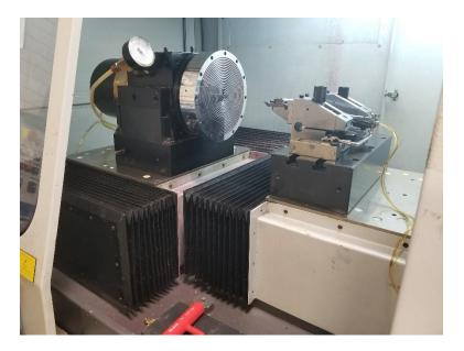
Figure 4.10 Precitech 350 diamond turning machine
