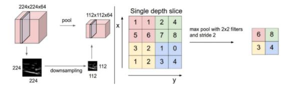
Figure 2.6: Max-Pooling Layer <sup>2</sup>
