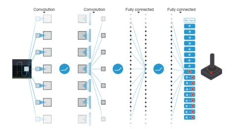
Figure 2.4: Deep Q Network Convolutional Neural Network Architecture [3]
