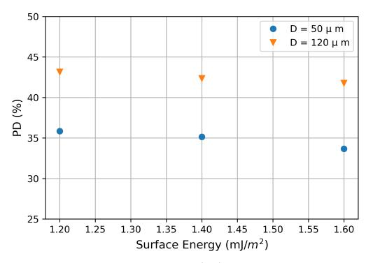
Figure 5.13: Packing density (PD) against surface energy.
