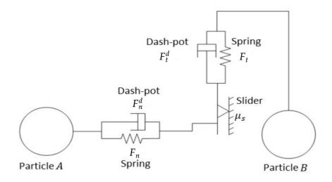
Figure 3.4: Hertz-Mindlin Contact Model [2].
