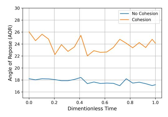
Figure 5.17: Angle of repose (AOR) with and without cohesion.
