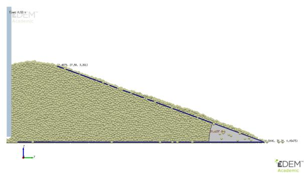
Figure 5.16: Angle of repose (AOR) setup.
