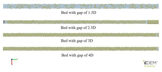
Figure 5.11: Powdered bed for different Gap size.
