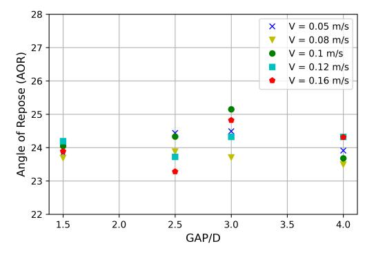
Figure 5.18: Angle of repose (AOR) against Gap/D and different velocities.
