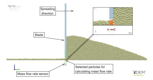
Figure 5.1: Mass flow rate (MFR) calculation setup.
