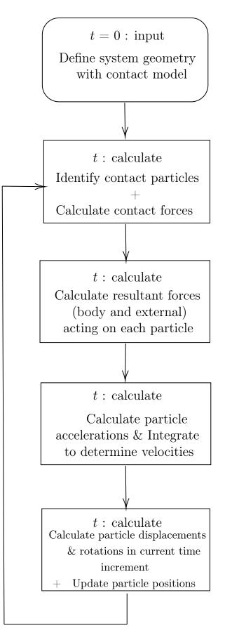
Figure 2.2: The general algorithm used in DEM calculations. [18]
