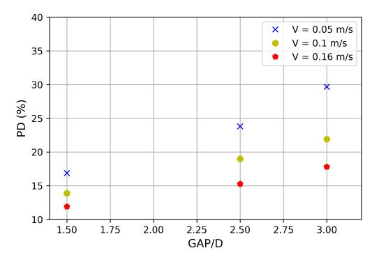
Figure 5.10: Packing density (PD) against Gap/D and different velocities and COR.
