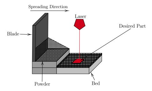
Figure 1.1: Selective Laser Sintering Process Layout.
