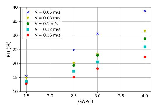
Figure 5.7: Packing density (PD) against  $\operatorname{Gap}/D$  and different velocities.
