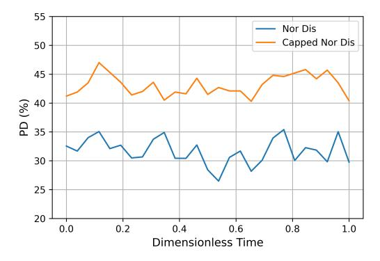
Figure 5.14: Packing density (PD) against capped and uncapped normal distribution.
