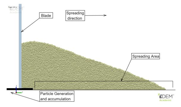
Figure 4.1: Simulation Setup.
