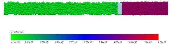
Figure 5.8: Particle velocities after spreading for blade speed 0.05 m/s.
