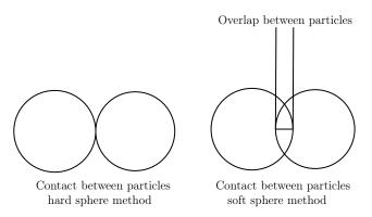
Figure 2.1: Hard and soft sphere contacts.
