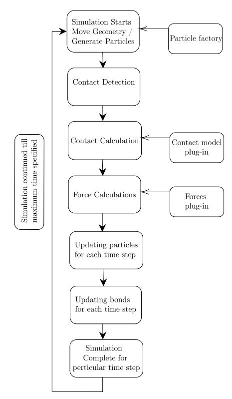
Figure 3.1: Simulation / Calculation Sequence in  $EDEM^{TM}$  [1].
