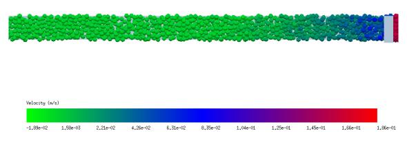
Figure 5.9: Particle velocities after spreading for blade speed 0.16 m/s.
