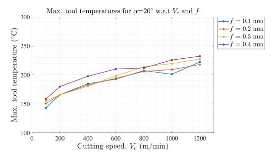
Figure 5.18: Variation of maximum tool temperatures with cutting speeds and uncut chip thickness at  $\alpha = 20^{\circ}$ .
