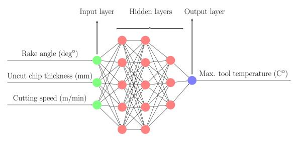
(b) Example of a deep neural network predicting maximum tool temperature.
