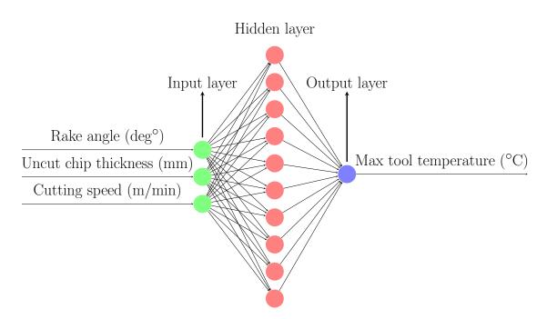
(b) Example of a shallow neural network predicting maximum tool temperature.
