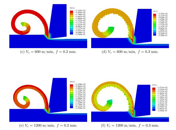
Figure 5.19: Temperature profiles obtained from FEA simulations for rake angle  $\alpha = 8^{\circ}$ , uncut chip thickness f = 0.2 mm and 0.3 mm at cutting speeds  $V_c = 400$  m/min, 600 m/min and 1200 m/min respectively.
