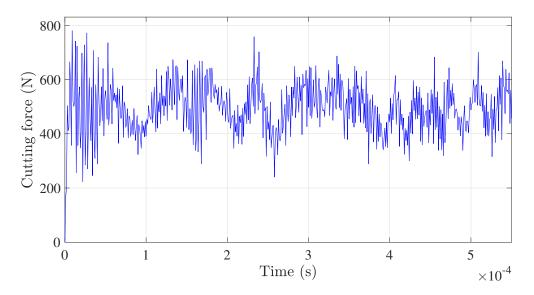
Figure 5.1: Cutting forces for  $V_c = 600 \text{ m/min}$ ,  $\alpha = 15^{\circ}$  and f = 0.2 mm obtained from FEA simulations.
