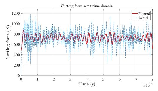
Figure 5.5: Actual cutting force and filtered cutting force.
