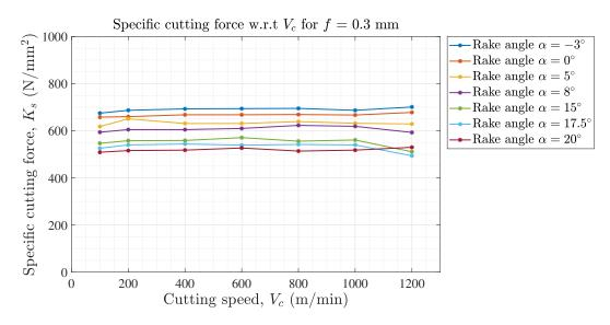
Figure 5.10: Variation of specific cutting forces with cutting speeds and rake angles at f = 0.3 mm.
