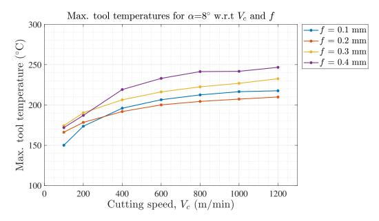
Figure 5.15: Variation of maximum tool temperatures with cutting speeds and uncut chip thickness at  $\alpha = 8^{\circ}$ .
