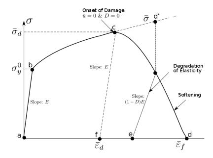
Figure 3.4: Stress-strain curve for material undergoing damage.
