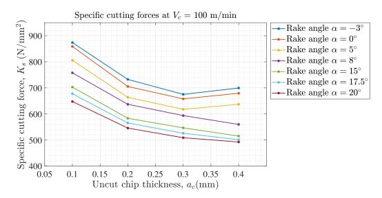
Figure 5.6: Variation of specific cutting forces with uncut chip thickness and rake angles at  $V_c = 100$  m/min.
