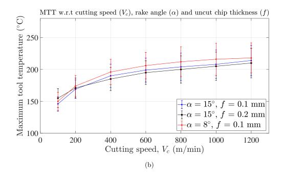
Figure 7.6: Specific cutting forces (7.6a) and maximum tool temperature (7.6b) obtained from FEA simulations.
