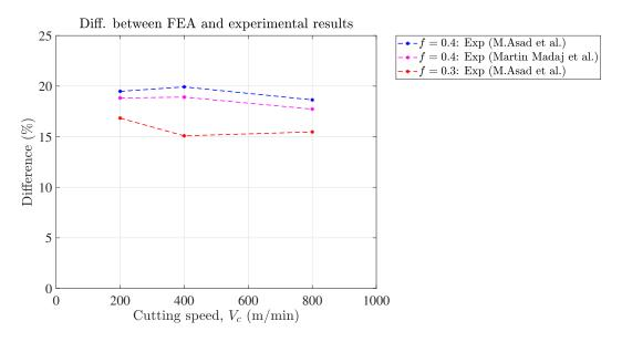
Figure 4.2: Difference in specific cutting forces.
