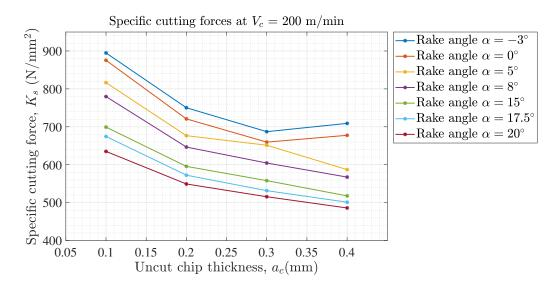
Figure 5.7: Variation of specific cutting forces with uncut chip thickness and rake angles at  $V_c = 200$  m/min.
