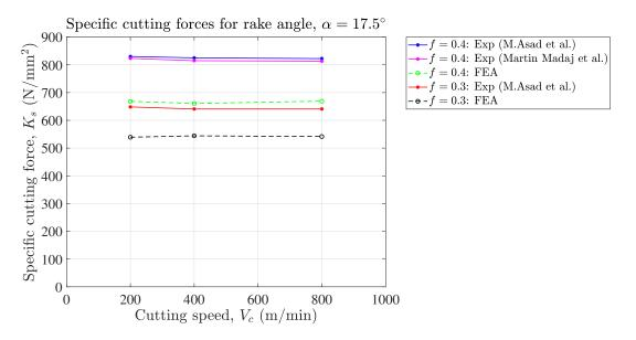
Figure 4.1: Comparison of FEA specific cutting forces with experimental results.
