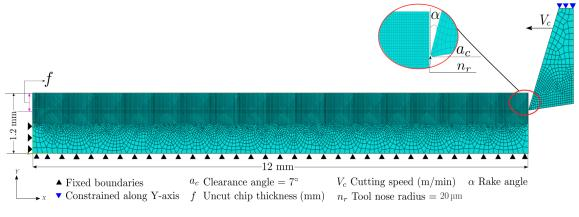
Figure 3.2: Finite element model setup.
