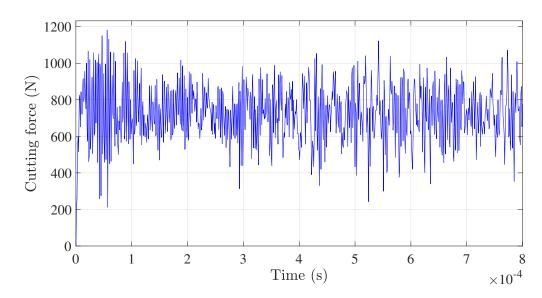
Figure 5.2: Cutting forces for  $V_c = 400$  m/min,  $\alpha = 8^{\circ}$  and f = 0.3 mm obtained from FEA simulations.
