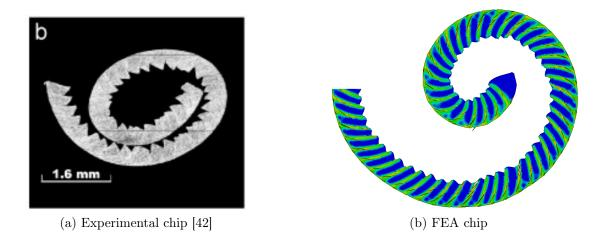
Figure 4.3: Comparison of chip shape obtained from FEA simulations (4.3b) with physical chip obtained from machining experiments (4.3a).
