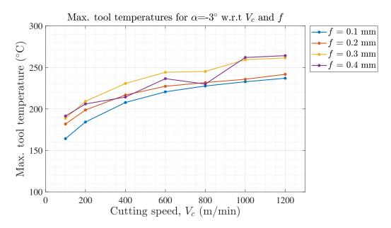
Figure 5.12: Variation of maximum tool temperatures with cutting speeds and uncut chip thickness at  $\alpha = -3^{\circ}$ .
