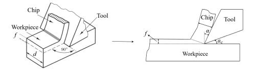
Figure 1.1: Orthogonal machining [2].
