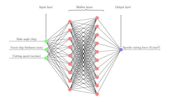
Figure 7.3: Suitable deep neural network with architecture 3-9-10-0-1 for predicting specific cutting forces.
