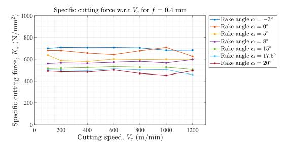
Figure 5.11: Variation of specific cutting forces with cutting speeds and rake angles at f = 0.4 mm.
