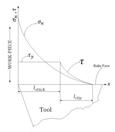
Figure 3.3: Normal stress  $\sigma_n(x)$  and shear stress  $\tau$  distribution at the tool rake face as per Zorev's friction model [4].
