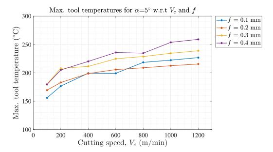
Figure 5.14: Variation of maximum tool temperatures with cutting speeds and uncut chip thickness at  $\alpha = 5^{\circ}$ .
