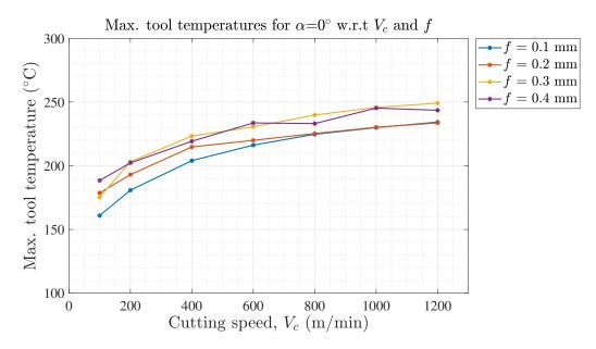
Figure 5.13: Variation of maximum tool temperatures with cutting speeds and uncut chip thickness at  $\alpha = 0^{\circ}$ .
