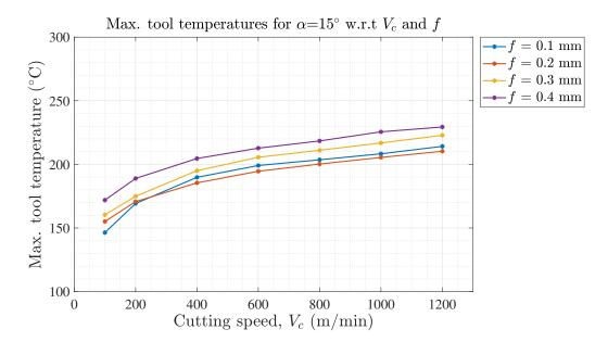
Figure 5.16: Variation of maximum tool temperatures with cutting speeds and uncut chip thickness at  $\alpha = 15^{\circ}$ .
