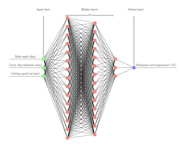
Figure 7.1: Suitable deep neural network with architecture 3-15-14-3-1 for predicting maximum tool temperatures.
