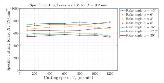
Figure 5.9: Variation of specific cutting forces with cutting speeds and rake angles at f = 0.2 mm.
