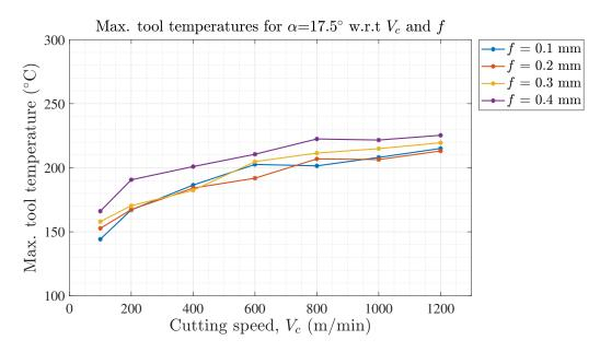
Figure 5.17: Variation of maximum tool temperatures with cutting speeds and uncut chip thickness at  $\alpha = 17.5^{\circ}$ .
