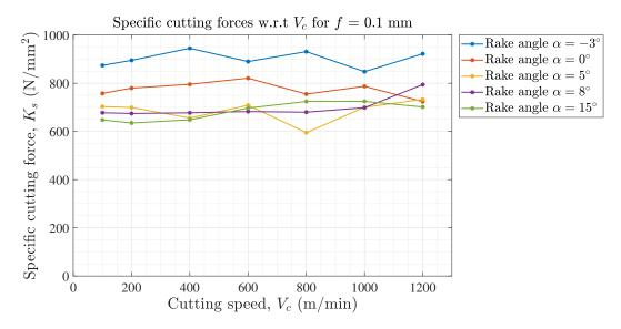
Figure 5.8: Variation of specific cutting forces with cutting speeds and rake angles at f = 0.1 mm.
