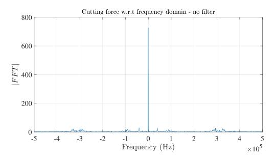
Figure 5.3: Fast Fourier transform for the cutting forces shown in Figure 5.2.
