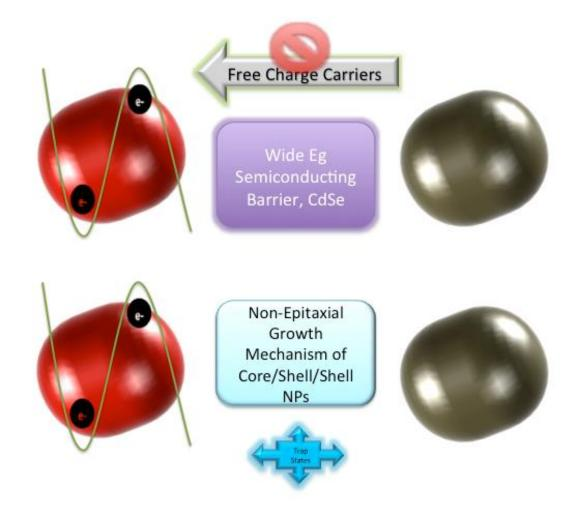
Figure 34: Vital aspects to ensure that this approach worked. The wide bandgap spacer (purple = CdX) was placed to minimize energy loss into the metal. We chose a non-epitaxial growth mechanism of the core/shell/shell NPs to minimize the defects that act as trap states.
