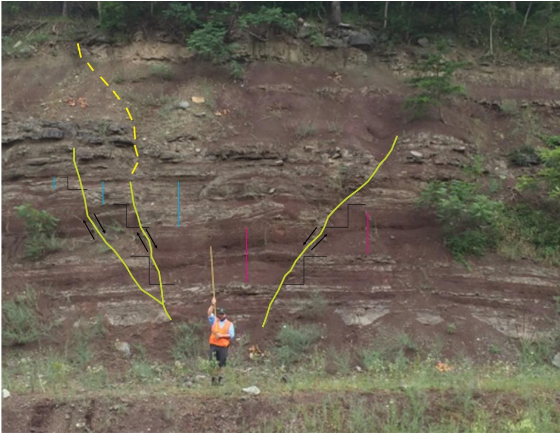
Figure 75: Alternative interpretation of the horst and graben near the eastern extent of the southern outcrop. The yellow lines indicate observed faults, the arrows indicate movement direction, and the black lines correlate units on both sides of the faults. The dashed yellow line at the top of the outcrop indicates possible continuation of a fault to the top of the section. The blue lines show decreasing sandstone unit thickness moving out of the graben, while the pink lines show decreasing siltstone unit thickness moving out of the graben. Note that the location of the uppermost part of the fault (dashed line) coincides with the pinch out of the thick-bedded sandstone (facies association 3) at the top of the exposure. This implies that growth-faulting may have created contemporary topographic lows that influenced the position of the thick-bedded sandstone (facies association 3). Field assistant for scale (about 1.75 meters tall).
