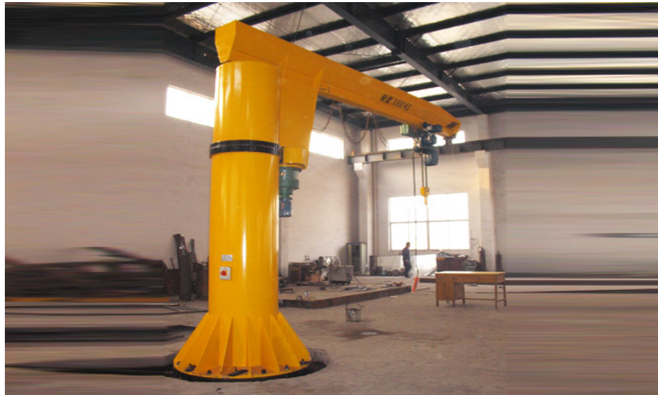
FIGURE 2: Fixed jib crane Source: Fixed jib crane. (2014).
