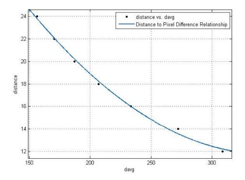
Figure 5.10: Pixel spacing to distance curve fitting
