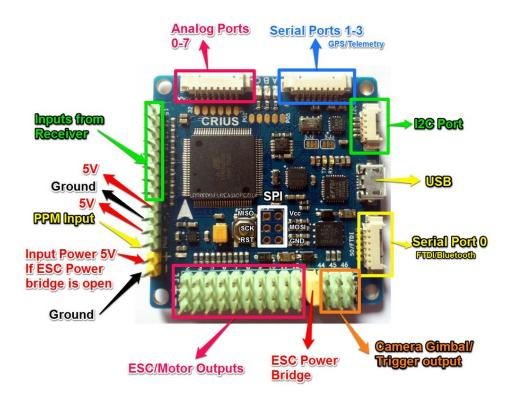
Figure 3.3: Diagram of Crius AIOP v2 [3]
