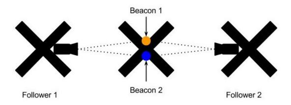
Figure 5.1: Example formation for color detection based vision system
