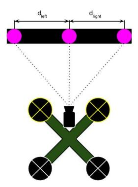
Figure 5.3: Distance measurement between quadrotor and beacon
