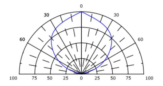
Figure 5.8: Characteristics of individual infrared LED angle vs. intensity [13] 30° at a distance of 18 inches.
