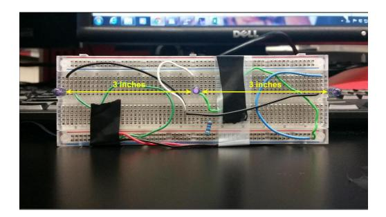
Figure 3.5: Prototype infrared beacon
