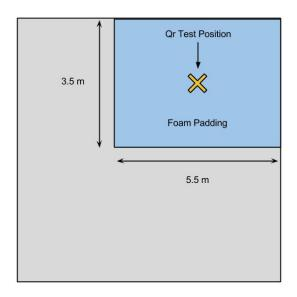
Figure 4.1: Illustration of safe quadrotor flight testing environment
