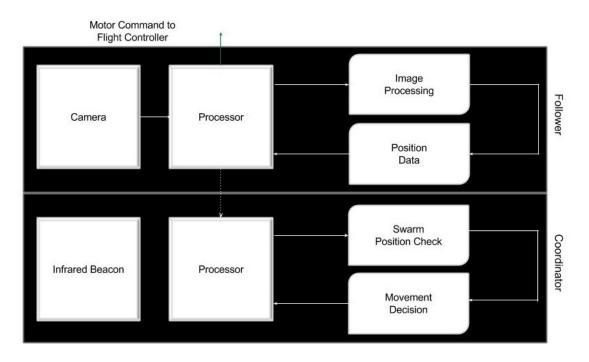
Figure 3.2: High-level flow diagram for interaction between coordinator and follower
