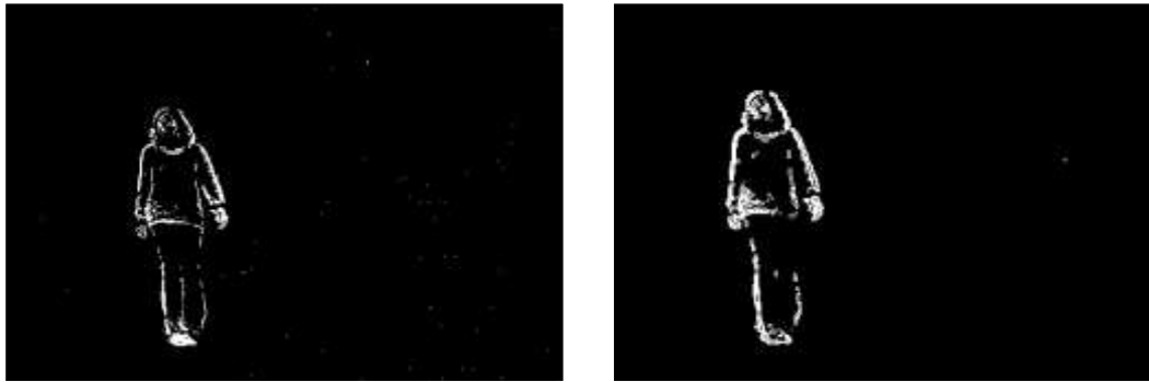
Figure 4: Effect of using the Wiener Filter. The original is on the left
