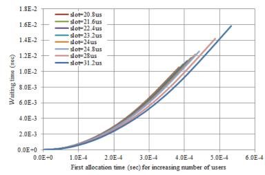
Figure 34: First allocation time dependence on number of users and associated waiting time. Note that this only shows the first phase in bandwidth allocation which is done by allocating based on user weightage
