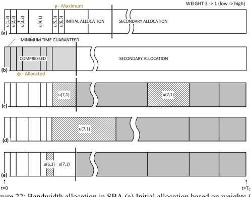
Figure 22: Bandwidth allocation in SBA (a) Initial allocation based on weights (b) Secondary allocation (c) Secondary allocation for user 7 (d) Efficient single combined slot for user 7 (e) Secondary allocation for user 6. Initial allocation (left of bold vertical line) and secondary allocation (right of bold vertical line)
