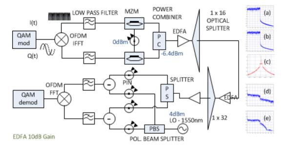
Figure 7: Component level view of proposed architecture. Transmitter: (a) OFDM signal generated after IFFT using NSC subcarriers, non-filtered, 25GHz (b) Filtered output of OFDM to be modulated onto the optical carrier at 1550nm. Roll-off of 0.5 and cut-off set at 0.62. Link: (c) Transmitted optical signal with modulated OFDM signal. Receiver results (d) down converted in-Phase signal at the receiver (e) signal after passing through raised cosine low pass filter. BER of 5.4 \* 10-3 (Figure 10).
