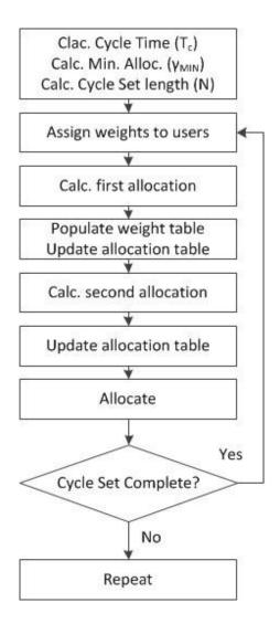
Figure 24(a): Flow chart for allocation in SBA
