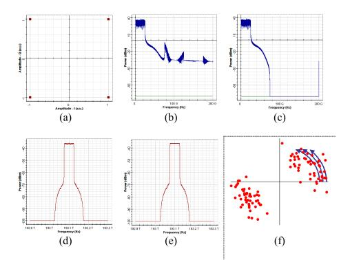
Figure 8: Coherent 100Gb/s transmitter with 2bits/symbol. (a) Constellation Diagram
