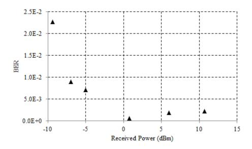
Figure 11: Received signal power and its effect on BER performance for the 16-QAM OFDM signal. With two amplifiers connected in tandem between the splitters we get reasonable BER.
