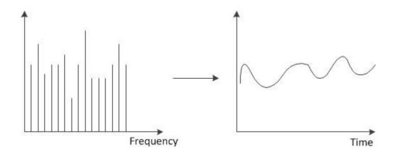
Figure 2: OFDM sub-carriers (frequency domain) to time-domain signal
