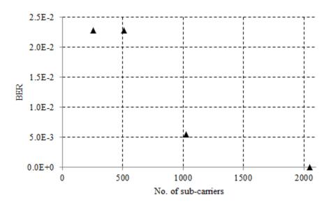
Figure 10: Effect of increasing the number of subcarriers on BER. Increasing number of sub-carriers increases bit error rate significantly but shows unpredictable dependence.
