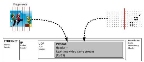
Figure 13: UDP/IP protocol stack on Ethernet channel
