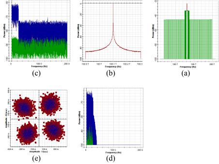
Figure 9: 100Gb/s receiver (a) Incoming signal spectrum (b) Local Oscillator 193.1 THz -2dBm (c) Limiting Amplifier (d) bandwidth limited signal (e) Received Optical Signal RED = Signal BLUE = noise
