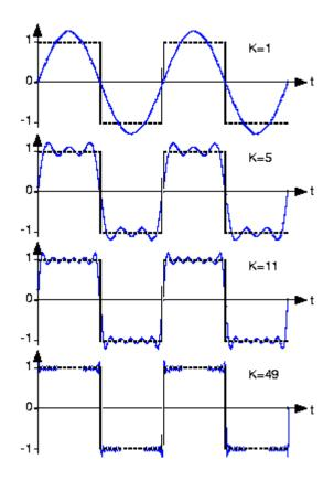
Figure 4: A square wave generated with multiple sine waves [38]
