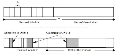
Figure 21: Cycle time distribution in RC-DBA. Pre-allocation state (top) and postallocation state (bottom)
