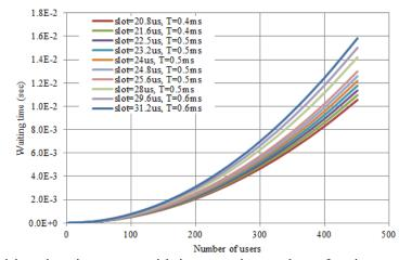
Figure 33: Waiting time increases with increase in number of active users. Various slot times and corresponding cycle times are plotted for a better view of system latency
