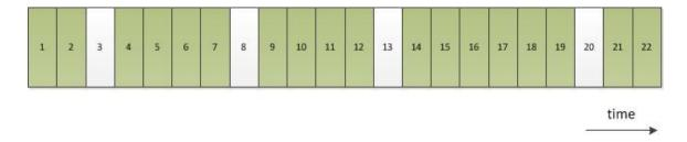
Figure 5: Typical time division multiplexing (TDM) allocation cycle
