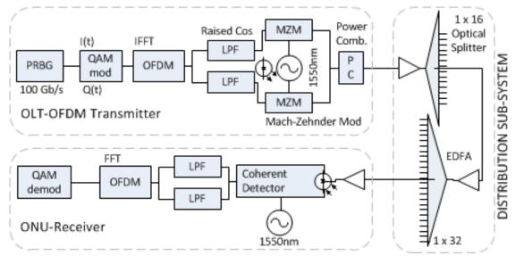
Figure 6: Block Diagram of proposed architecture. Three major components are the OFDM transmitter, distribution system and the OFDM receiver
