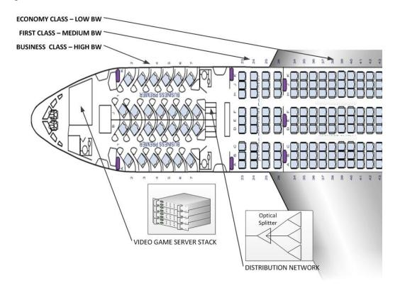
Figure 1: System Deployment – Optical network based architecture for in-flight systems (adapted from flight schematic) [13]
