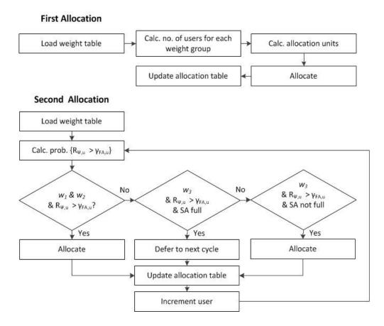
Figure 24(b): Flow chart: first and second allocation
