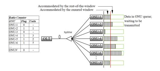
Figure 20(a): An overview of RC-DBA ratio counter and allocation table
