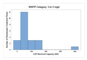
Figure 6-3: Histogram of WWTP CHP Electrical Capacities for WWTPs with Average Flows of 1 to 5 Mgd
