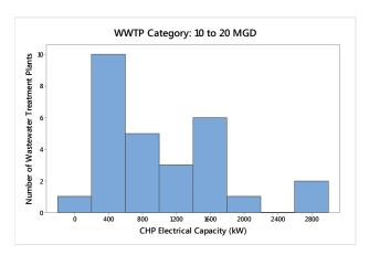
Figure 6-5: Histogram of WWTP CHP Electrical Capacities for WWTP with Average Flows of 10 to 20 Mgd
