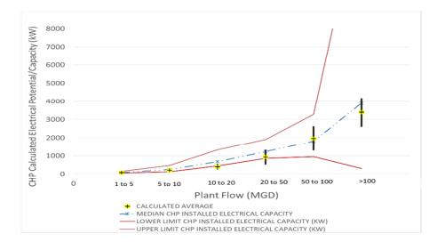
Figure 6-9: Wastewater Flow versus Actual and Calculated Electrical Capacities
