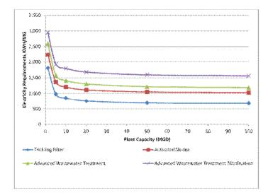
Figure 6-1 Electricity Demand for Wastewater Treatment by Size of Plant and Treatment Type Source: EPRI (2002)
