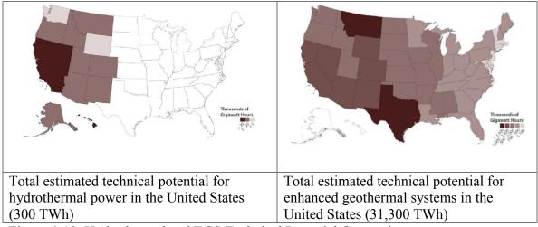
Figure 4-18: Hydrothermal and EGS Technical Potential Comparison Source: (Lopez et al., 2012)
