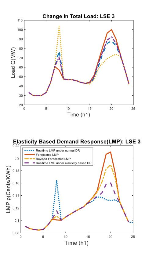
Figure 5.14: Surge mitigation (Load and LMP) under elasticity based forecasted rates (LSE 3)
