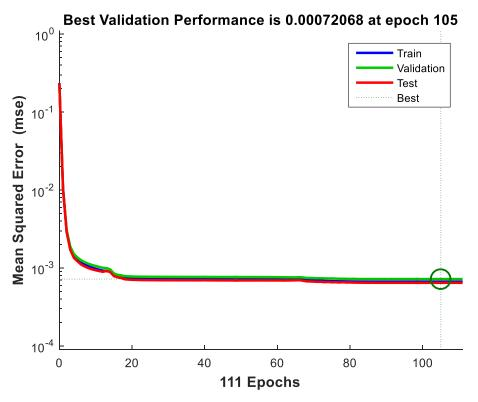
Figure 4.4: Performance plot indicating mean square error during traing validation and testing phase
