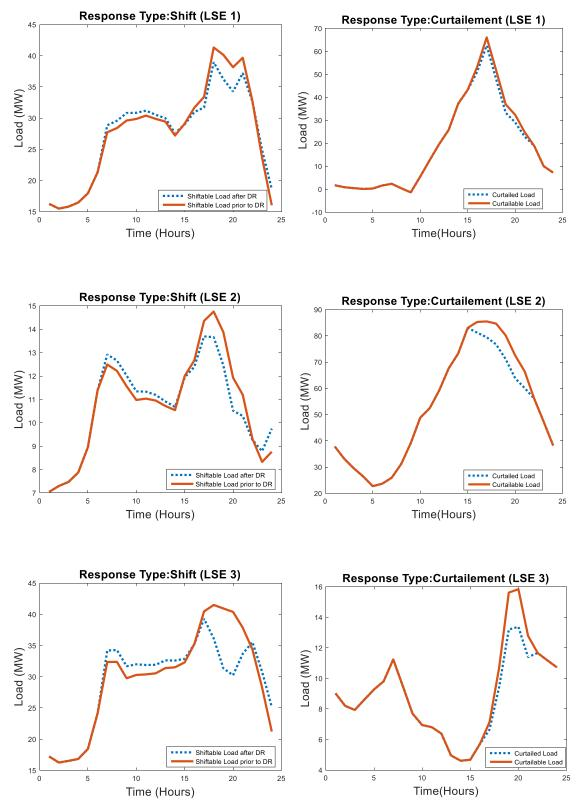
Figure 4.17: Curtailment and shift type reponse based on Consumer Psychology Model (Scenario 1)
