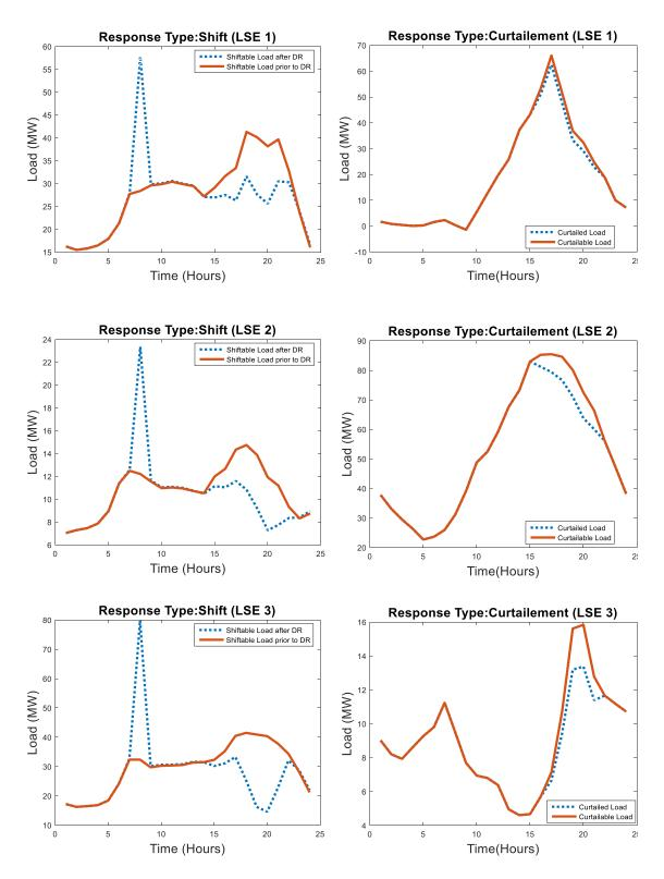
Figure 4.20: Curtailment and shift type reponse based on Consumer Psychology Model (Scenario 2)
