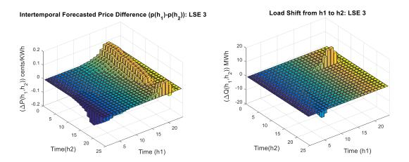
Figure 4.19: Benefit factor and corresponding load shift (Scenario 2)
