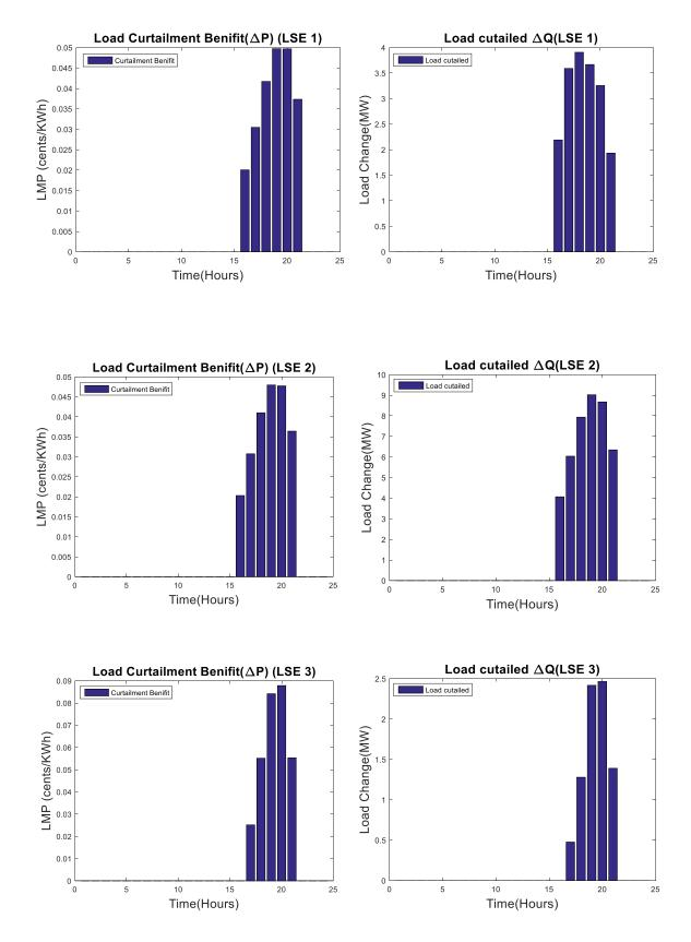
Figure 4.15: Benefit factor and corresponding load curtailment
