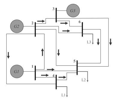
Figure 2.1: Test System: 6 Bus
