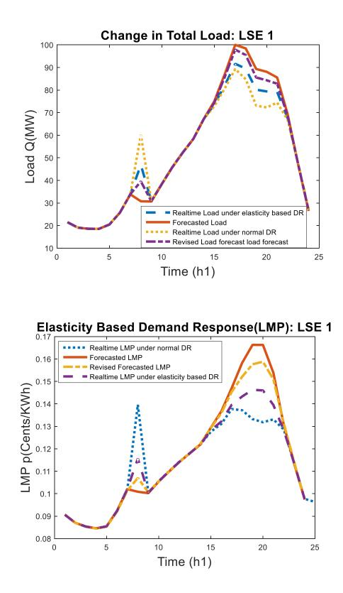
Figure 5.12: Surge mitigation (Load and LMP) under elasticity based forecasted rates (LSE 1)
