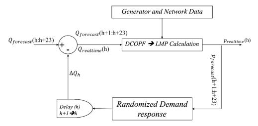
Figure 3.1: Closed loop demand response architecture
