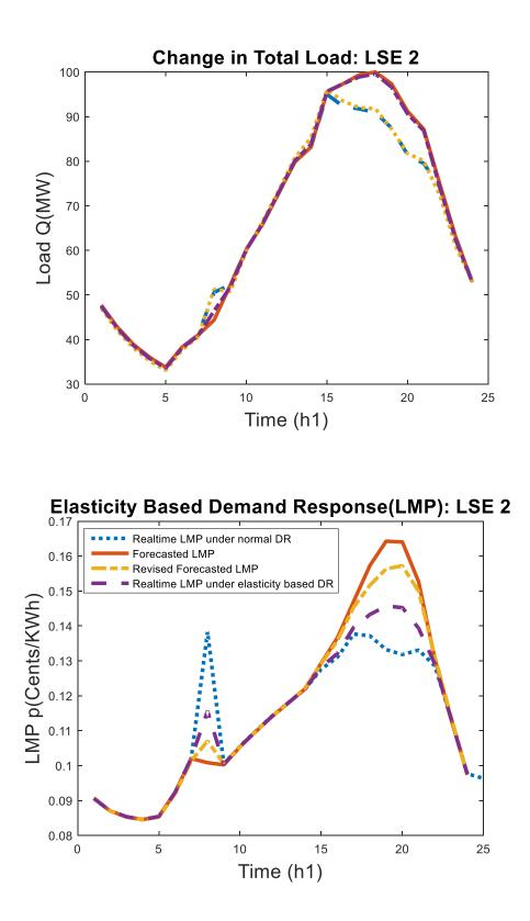
Figure 5.13: Surge mitigation (Load and LMP) under elasticity based forecasted rates (LSE 2)
