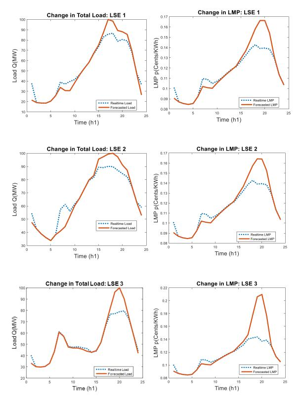
Figure 3.2: Load change and corresponding LMP change for 3 LSEs based on probabilistic demand response model
