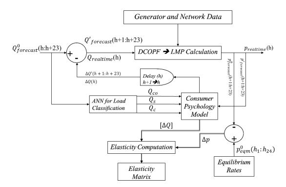
Figure 5.2: Architecture for estimating elasticity
