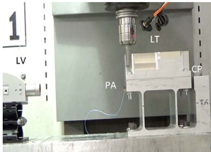
Figure 5.6: Milling experimental setup with laser vibrometer (LV), low mass piezo-accelerometer (PA), laser tachometer (LT), and capacitance probe (CP).
