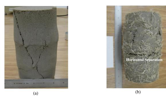
Figure 4.12: Typical Failures: (a) Angular Shear; (b) Bulging with Horizontal Separation
