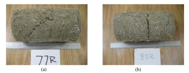
Figure 4.14: 10% Kaolin Clay-90% Ottawa Sand Specimen: (a) 1.5% Fiber Angular Failure Surface; (b) 1.75% Fiber Bulging Failure Surface
