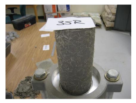
Figure 3.14: Test Specimen Extruded Successfully without Issues
