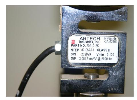
Figure 3.17: Load Cell Used During the UC Testing
