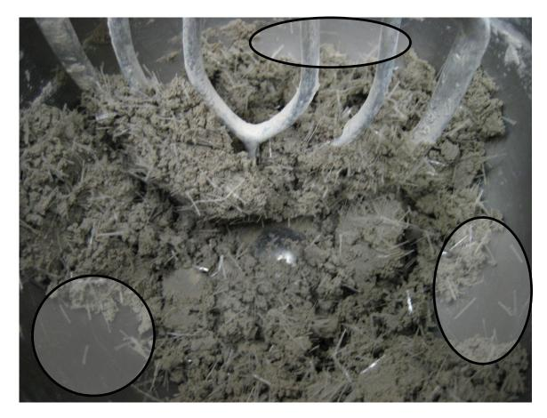
Figure 3.12: Fibers Adhering to the Side of the Mixing Bowl
