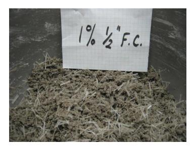
Figure 3.11: Fibers Floating on Top of the Soil
