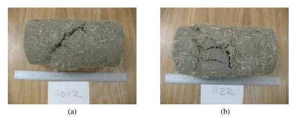
Figure 4.15: 15% Kaolin Clay-85% Ottawa Sand Specimen: (a) 1.25% Fiber Angular Failure Surface; (b) 1.5% Fiber Bulging Failure Surface
