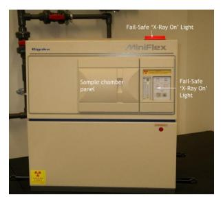
Figure 3.18: Rigaku Miniflex+ XRD
