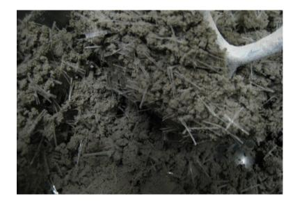
Figure 3.10: Final Soil Mix after the Addition of Fiber Reinforcement
