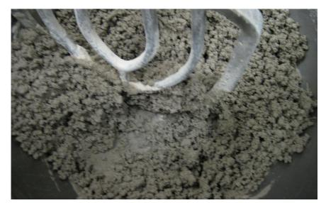
Figure 3.9: Mixed Kaolin Clay-Ottawa Sand Soil Beginning to Cohere
