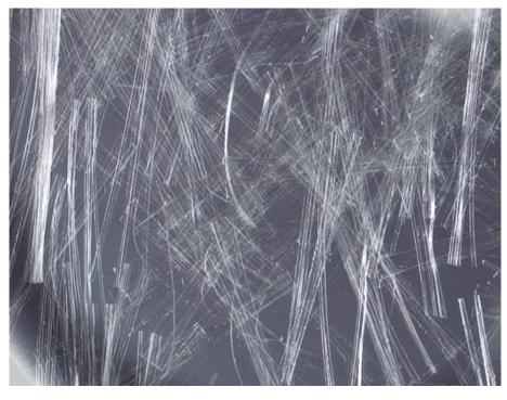
Figure 3.5: FIBERCAST 500<sup>™</sup> Polypropylene Fibrillated Fiber
