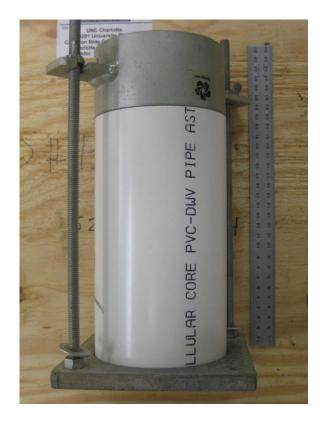
Figure 3.6: Custom Compaction Mold Used to Generate the Test Specimens
