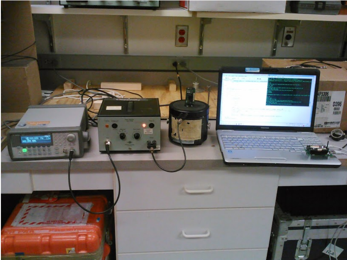
Figure 3.2.3: Shaker and Accelerometer Calibration Setup
