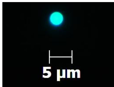
FIGURE 3: Fluorescent microscopy image of 3µm bead viewed at 400x using the Zeiss filter set 25(ex. 400+495+570, em. 460+530+625)
