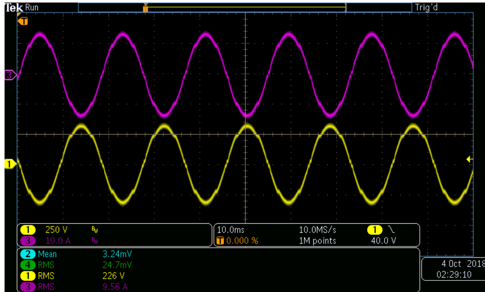
(a) Yellow: Output voltage, Pink: load current
