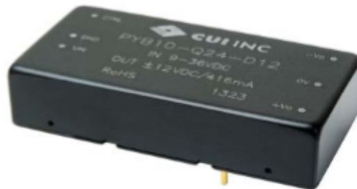
(a) 24V-15V power supply for PV and BESS board
