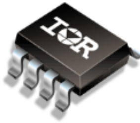
Figure 4.4: Self oscillating half bridge driver
