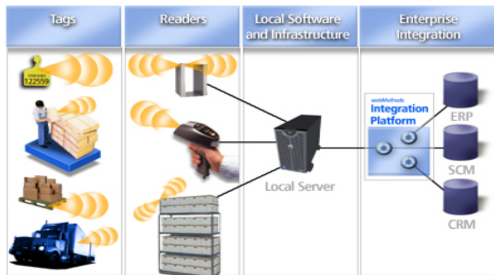
Figure 1: An RFID System in Retail Supply Chain Source ( http://www.foodylife.com )
