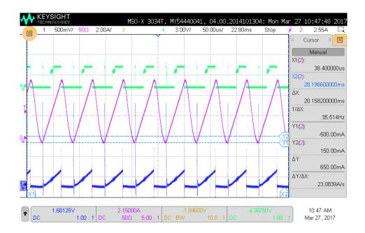
Figure 7.10: **Experimental results**: SenseGaN operation at 2.5A with 350mV/A sensitivity. Purple: inductor current measurement (amplifier current gun), Blue: SenseGaN measurement, Green: generated trigger signal from the analogue comparator (TLV3502).
