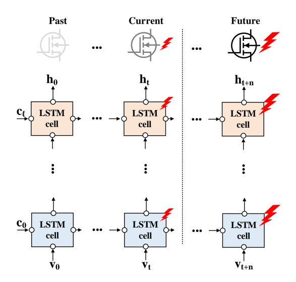
Figure 4.7: The stacked LSTM: An unrolled LSTM cell predicts the next n samples of  $\Delta R_{ds(on)}$  based on last sensed data.
