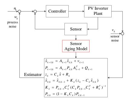
Figure C.4: **Self-healing scheme**: The proposed scheme for modified model of the PV inverter system considering the sensor characteristics and Kalman filter estimator.
