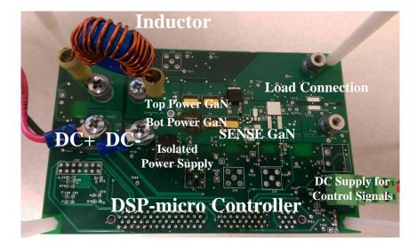
Figure 7.4: **Hardware setup**: The prototype was designed in four layers: Top layer: Power stage, Inner layer-1: Power ground, Inner layer-2: Shield layer, Bottom layer: Control signals and conditioning circuits.
