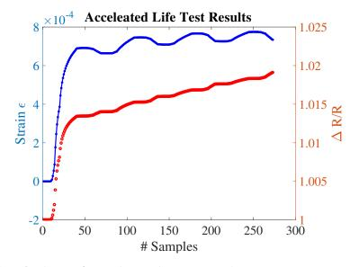
Figure 3.7: Simulation of strain-resistance: The resistance variations and the strain changes are simulation based on the proposed geometry.
