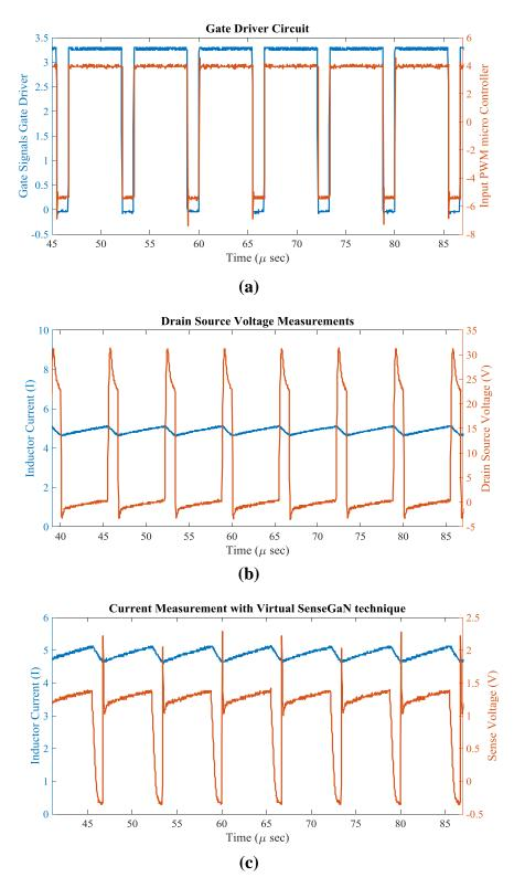
Figure 7.5: **Experimental results**: a) blue: input gate signal from micro controller, and orange: output gate signals of the isolated gate driver. b) blue: inductor current measured with amplifier current gun, orange: drain-source voltage of the converter c) blue: inductor current measured with amplifier current gun, orange: current gun, orange: current measurement with SenseGaN 150kHz, 5A boost power converter.
