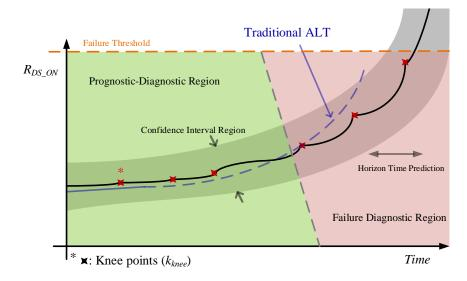
Figure 3.2: **Proposed solution**: Adaptive prognostics concept using multi-physics co-simulations and machine learning algorithm with advanced monitoring.
