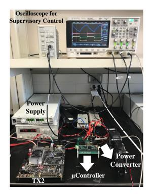
Figure 6.9: **Experimental verification**: The hardware setup was implemented including the high-frequency power converter controller by  $\mu$ -controller, the SoC-TX2 for edge computation. The supervisory control is designed for the safety protection.
