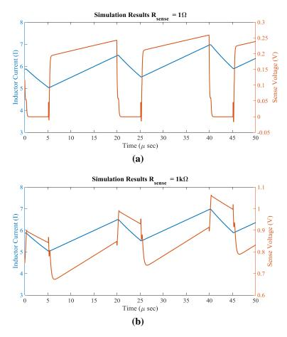
Figure 7.3: Spice simulation results: SenseGaN in two different scenarios. blue: inductor current, orange: measurement with SenseGaN circuit a) sensing resistor is  $1\Omega$ , b) sensing resistor is  $1k\Omega$ . As it shown choosing higher resistance would impact the sensing significantly. For these devices, it is recommended to use sensing resistor  $<20\Omega$  to compromise between higher efficiency and system robustness performance.
