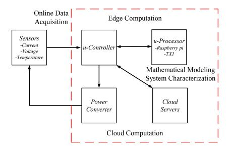
Figure 6.1: The proposed reliability solution: The advanced solution leverages the benefits of Internet of Things for reliability analysis using edge/cloud.
