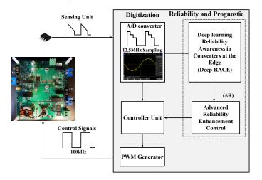
Figure 5.1: The edge node diagram: It consists of a  $\mu$ -controller and AI SoC to generate gate signals and predict the trajectory resistance of power transistor.
