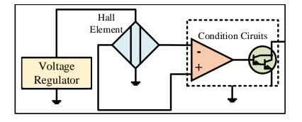
Figure C.3: **Current sensor model**: The scheme of Hall-Effect current sensor for age modeling.
