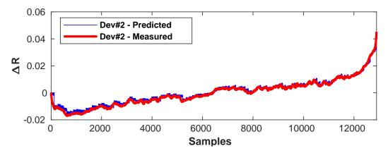
Figure 6.3: **Experimental results:** The prediction of  $\Delta R_{ds(on)}$  variations of device-2 through Deep RACE method.
