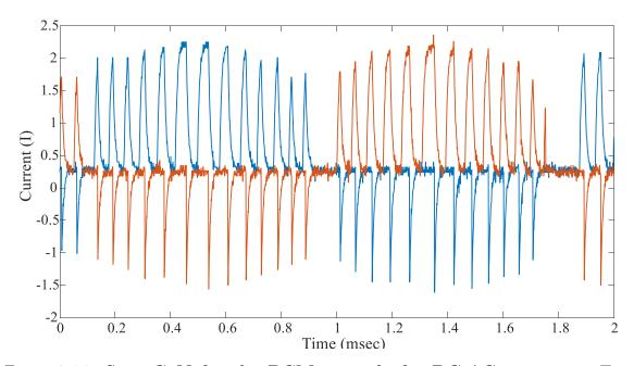
Figure 7.24: SenseGaN for the BCM control of a DC-AC converter: Two reference trigger signals are considered to turn-on the bottom devices consecutively. The closed loop operation of the DC-AC converter operation is verified in CHIL (top: bottom SenseGaN-1, orange: bottom SenseGaN-2)
