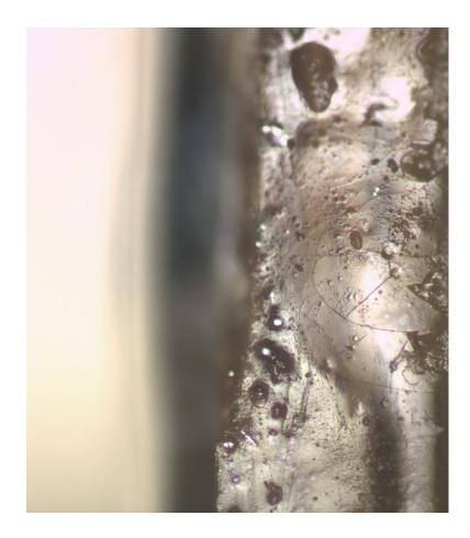
Figure 6.12: **Experimental results**: The solder degradation is observed on the source of GaN power devices in the defected device of the buck converter.
