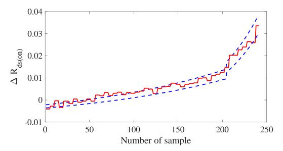
Figure 4.3: **Bayesian calibration**: The output results of the algorithm for pattern recognition within the confidence interval. Red: drain-source resistance changes, blue: the estimated resistance variation within the specific confidence level after the data filtering and highlighted near the knee point.
