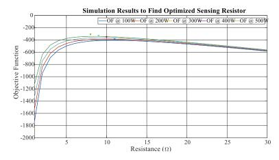
Figure 7.15: **Optimization in SenseGaN**: The compromise of higher performance (low resistance) vs. lower loss (high resistance) are analyzed in the OF.
