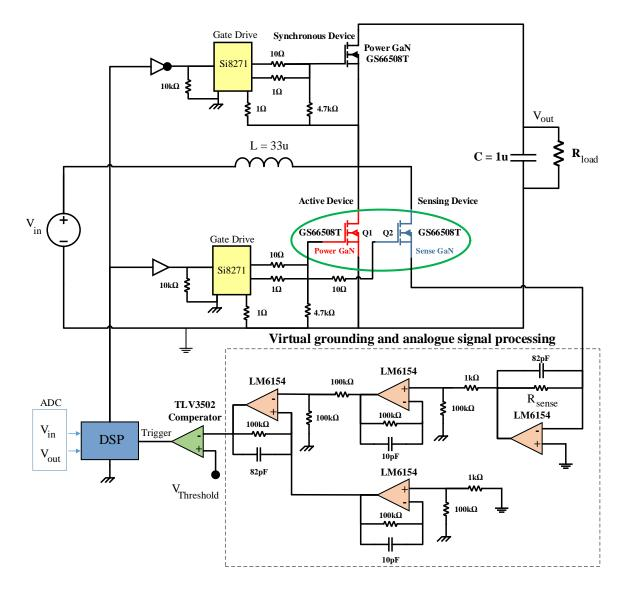
Figure 7.6: Schematic capture: The boost operation system with SenseGaN and control units.
