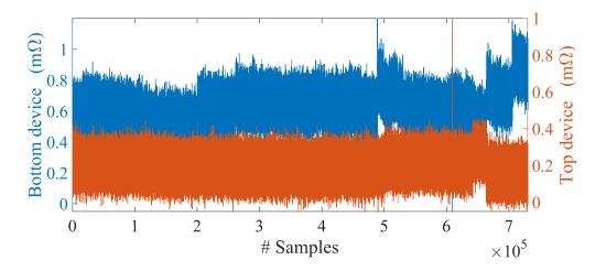
Figure 5.7: The filtered on-resistance variations: The buck converter was tested over 100 billion electrical cycles 400W and 100kHz. The drain-source on-resistance variations was captured automatically, and stored on the cloud networks.
