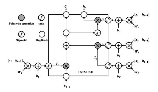
Figure 4.5: A single LSTM cell: Inside of an LSTM cell consisting of three gates and the state of the cell is preserved by variable  $c_t$ .
