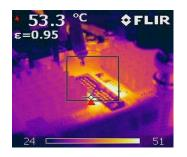
Figure 6.10: **Experimental verification**: Temperature rise control of the converter through thermal image.
