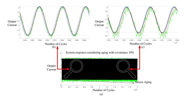
Figure C.5: **Simulation results**: The estimation results considered by a Kalman filter to the modified model of current sensor aging. The system response is modeled with 10% covariance error of the current sensor and shown based during the aging process. blue: ideal waveform, green: actual sensor measurement, red: system response correction with Kalman filter without aging considerations, black: system response correction with Kalman filter considering the aging process.
