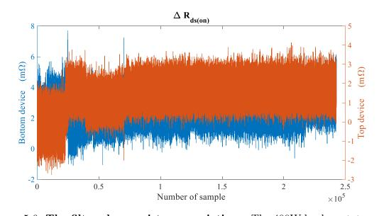
Figure 5.6: **The filtered on-resistance variations**: The 400W buck prototype was tested over 30G cycles with continuous operation at 100kHz switching frequency, and drain-source resistance variations was captured automatically.
