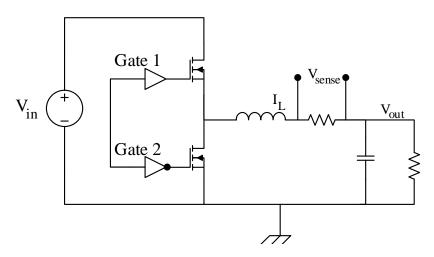
Figure B.1: Shunt method: Schematic of external sense resistor for capturing the inductor and output current. The voltage drop across the resistor theoretically can represent the actual current waveform; however, this method in practice has a lot of issues for high-frequency and high current applications.
