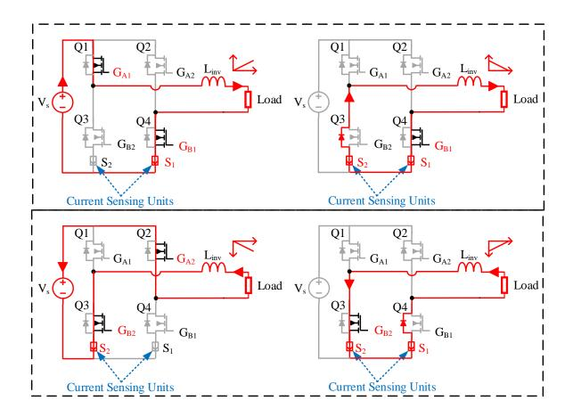
Figure 7.21: **Inverter operation**: The system operation for the BCM operation in the inverter, proposed by SenseGaN current mirroring techniques. The current path highlighted with red one shows the four modes of operation.
