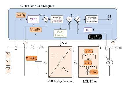
Figure C.1: **PV inverter schematic**: The proposed scheme for a single phase inverter with the control architecture
