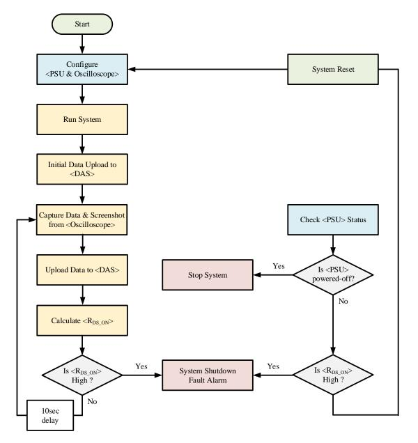
Figure 5.5: **Data acquisition system**: The thread is provided for device characterization and resistance measurement.
