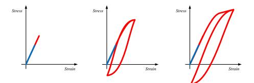
Figure 3.4: The hysteresis loss: Once the nominal mean stress is less than border mean stress (left) vs. the mean stress is higher than the border mean stress (right).
