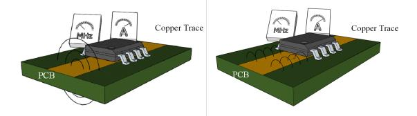
Figure B.4: Magneto-Resistors sensor: General operation of the contact-less AMR sensor: magnetic field generations at low frequency (left) and high-frequency (right) are shown.
