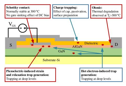
Figure 2.2: Lateral GaN structure: The most susceptible regions in GaN device.
