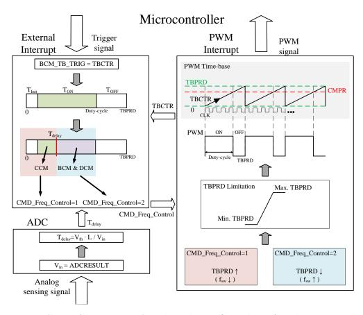
Figure 7.9: **SenseGaN control**: The scheme flow chart for the proposed BCM control algorithm.
