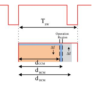
Figure 7.8: **The system operation modes**: The operational regions for distinguishing CCM, BCM, and DCM in a single cycle. Orange: CCM, Blue: Optimum region for BCM, Gray: DCM.
