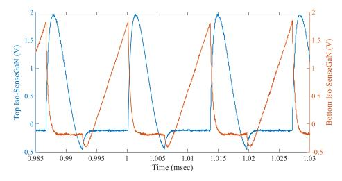
Figure 7.19: **BCM control of a DC-DC boost converter**: orange: bottom Iso-SenseGaN, blue: top Iso-SenseGaN outputs.
