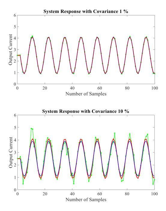
Figure C.2: Simulation results: The current sensor response under two different covariance measurement errors (1% and 10%). blue: ideal waveform, green: actual system reference response, red: modified system response correction with Kalman filter estimation.
