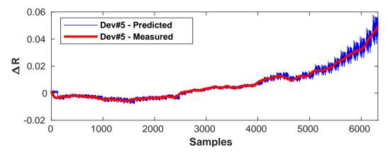
Figure 6.6: **Experimental results:** The prediction of  $\Delta R_{ds(on)}$  variations of device-5 through Deep RACE method.
