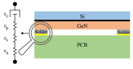
Figure 3.3: Mounted GaN on the PCB: Simplified model of a lateral GaN mounted on the PCB. GaN and Silicon (substrates) are isolated with thin layer of AlGaN, and packaging is not considered in the model.
