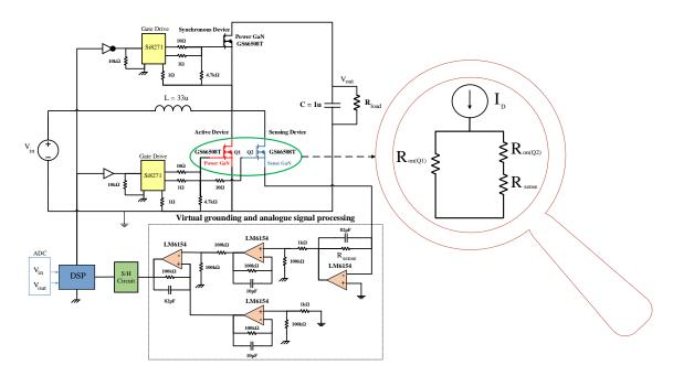
Figure 7.2: Schematic capture: Schematic of implemented virtual grounding for SenseGaN technique in a GaN boost converter. The virtual grounding circuit guarantee the tight connection of GaN power (Q1) and Sensing GaN (Q2) and consequently more accurate monitoring of the main current. The zoomed-in of the circuit shows the main current stream for temperature variation characterization.
