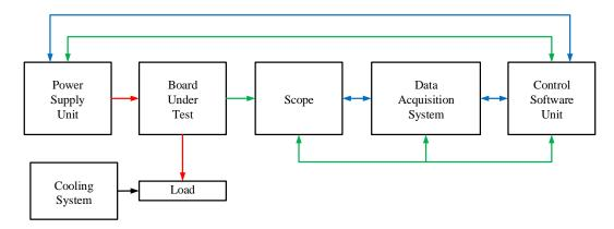
Figure 5.4: **Data acquisition system**: Supervisory system control was designed for data collection and converter protection. red: power path, blue: control signals, and green: sensing signals.
