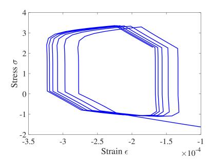
Figure 3.8: Simulation of strain-resistance: The simulated energy loss generated from the stress and strain variation of the joints in the accelerated life analysis.
