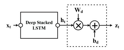
Figure 4.8: The proposed deep LSTM network model: A linear layer is added to the deep stacked LSTM to map  $h_t$  to on-line measured  $\Delta R$  at time t.
