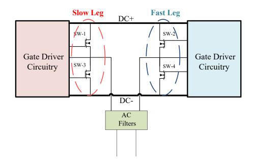
Figure A.1: Schematic configuration: The hybrid sinusoidal unipolar DC-AC converter topology considering one leg as fast switching, the second leg switching with grid frequency.
