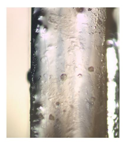
Figure 6.13: **Experimental results**: The solder degradation is not observed on the source and drain of GaN power devices in the healthy device of the buck converter.
