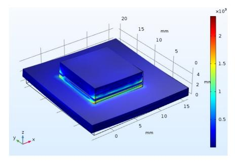
Figure 3.6: Simulation of the accelerated life test: The fatigue failure mode of the lateral GaN device is simulated through the finite element analysis.
