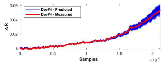
Figure 6.5: **Experimental results:** The prediction of  $\Delta R_{ds(on)}$  variations of device-4 through Deep RACE method.
