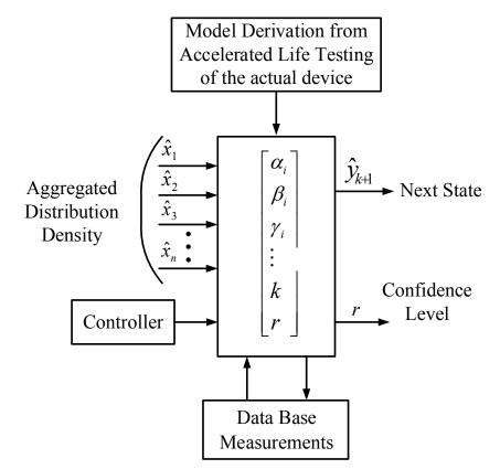
Figure 1.2: Conventional reliability modeling: Accelerated life tests of hundreds of hours are developed for extracting the mathematical modeling of device failure.
