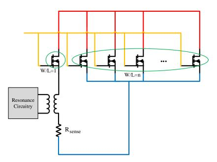
Figure 7.13: **Iso-SenseGaN**: The equivalent circuit model of the Iso-SenseGaN for the available lateral GaN.
