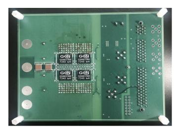
Figure 5.3: Hardware prototype: The buck converter designed in four layers.
