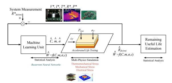
Figure 3.5: **Proposed framework for GaN power converter-Digital Twin**: The online device monitoring, and simulation-based ALT for reliability analysis. A machine learning system is developed for system calibrations and parameter estimations.
