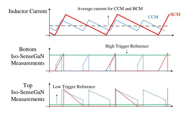
Figure 7.17: **BCM control of a DC-DC boost converter**: the current monitoring reflected in the Iso-SenseGaN. Two reference trigger signals are considered to turn-on the top and bottom devices consecutive.
