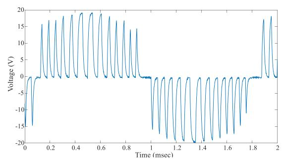
Figure 7.23: SenseGaN for the BCM control of a DC-AC converter: Two reference trigger signals are considered to turn-on the bottom devices consecutively. The closed loop operation of the DC-AC converter operation is verified in CHIL (blue: grid voltage)
