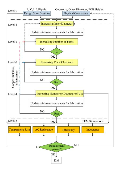
Figure A.2: **Optimization approach**: The algorithm descriptions to achieve the lowest resistance at the highest possible power density for the PCB embedded inductor within the 1-10MHz.
