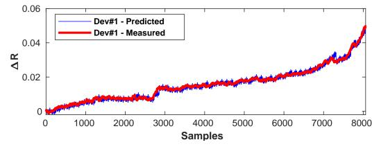
Figure 6.2: **Experimental results:** The prediction of  $\Delta R_{ds(on)}$  variations of device-1 through Deep RACE method.
