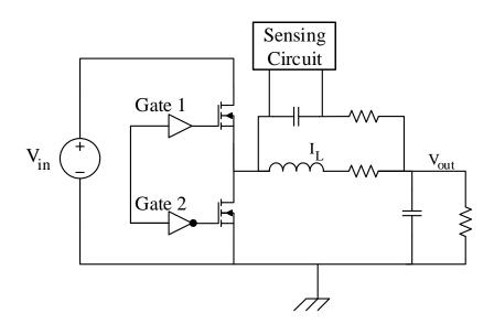
Figure B.3: Filter method: General schematic of filter-based current sensing. The active calibration for the passive element is required, and the common-mode voltage issue still exists in this approach.
