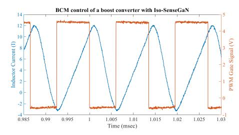
Figure 7.18: **BCM control of a DC-DC boost converter**: orange: PWM gate signals, blue: inductor current.
