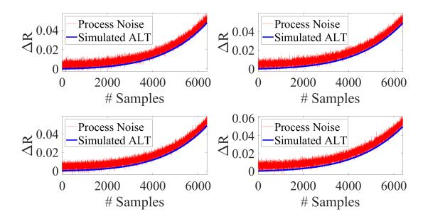
Figure 3.9: Simulation result of the accelerated life test: The variations  $R_{ds(on)}$  under temperature cycling due to solder fatigue of GaN on Silicon.
