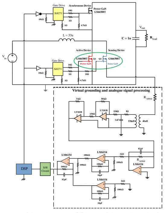
Figure 7.14: Schematic capture: a) Schematic of the virtual grounding for Iso-SenseGaN technique with galvanic isolation in a GaN boost converter.
