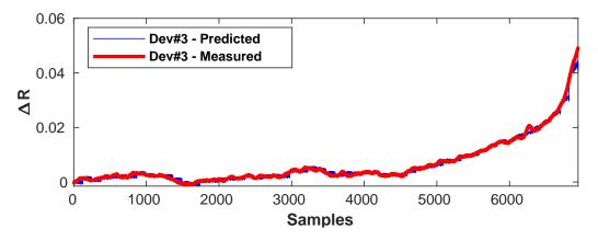
Figure 6.4: **Experimental results:** The prediction of  $\Delta R_{ds(on)}$  variations of device-3 through Deep RACE method.
