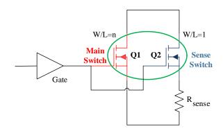
Figure B.2: **SenseFET**: General scheme of SenseFET. This technique should be implemented in an integrated package for higher performances.
