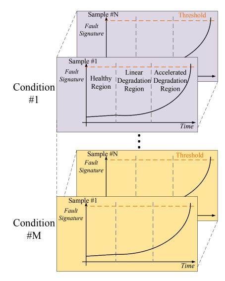
Figure 3.1: Conventional reliability solution: #N samples of devices with #M conditions have been analyzed experimentally under accelerated life tests to find the reliability model. Adaptability with the new technologies and the experimental costs are their main drawbacks.
