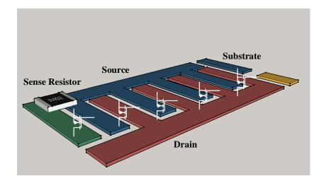
Figure 7.12: **Iso-SenseGaN configuration**: Proposing a scheme of Iso-SenseGaN for lateral dies based on available commercial products.
