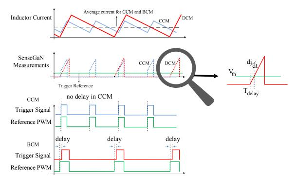
Figure 7.7: The system operation mode and curser identifications: a) The inductor current at CCM (blue) and BCM (red) with the same average current. b) The current monitoring with the SenseGaN for the active device in CCM and BCM. (here, the zoomed-in version of threshold trigger reference signal for delay generation is exposed) c) The microcontroller compares the trigger reference signal generated by the comparator and PWM signals to generate the delay signal in CCM and BCM.
