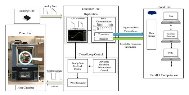
Figure 5.2: **New IoT approach for reliability assessment**: DAS for characterization of power converters, and multi-process computation on cloud networks. The proposed infrastructure architecture provides feasibility of data-processing techniques for adaptive prognostics in power electronics converters.
