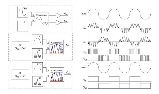
Figure 7.22: **Proposed BCM technique**: The analogue circuit logics for PWM generation through SenseGaN and the fundamental frequency of the grid.
