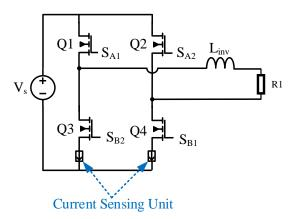
Figure 7.20: (Iso)SenseGaN for the BCM control of a DC-AC converter: The proposed architecture for the sensor placement in an inverter.
