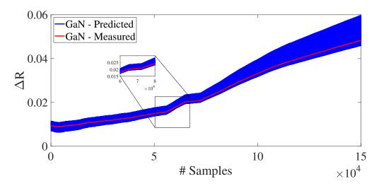
Figure 6.11: **Prognostic results**: The  $R_{ds(on)}$  variations for GaN with Si-substrate using the FEA simulations, and only one set of data for training.
